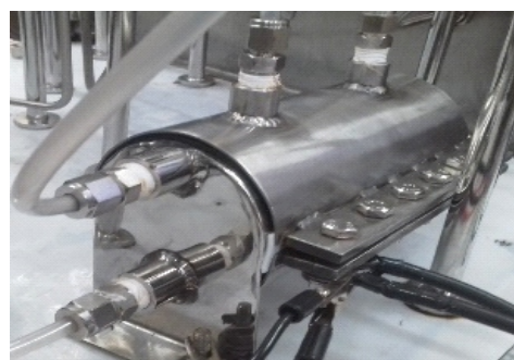
Cell for laboratory H_2 generator.
