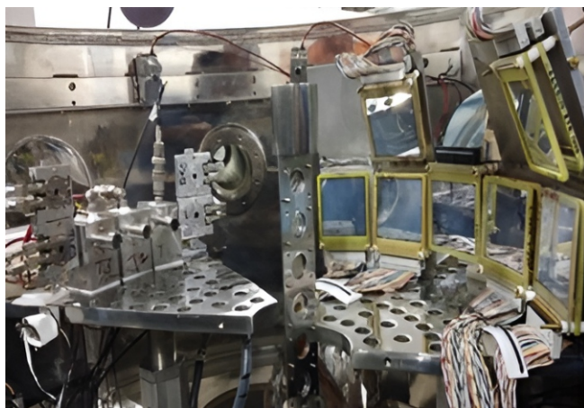
Fig.1: Typical detector setups inside the scattering chamber consisting of 5 sets of single telescopes and 7 (5) sets of strip telescopes, shown in left (right) panel, used for the breakup cross section measurements.
