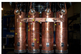
Assembly of four quarter wave resonators inside a cryostat.
