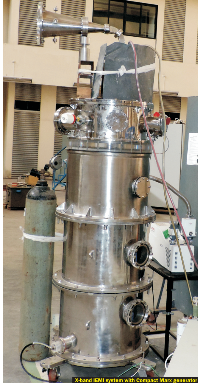
X-band IEMI system with Compact Marx generator
