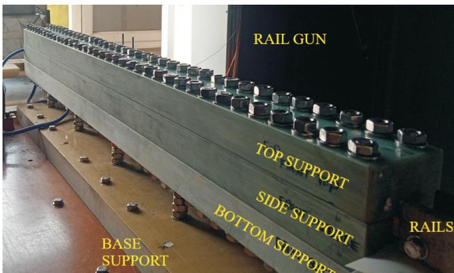
Fig.1: Electromagnetic railgun.
