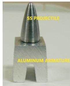
Fig.8: Projectile 316 SS with 7075 Al armature.
