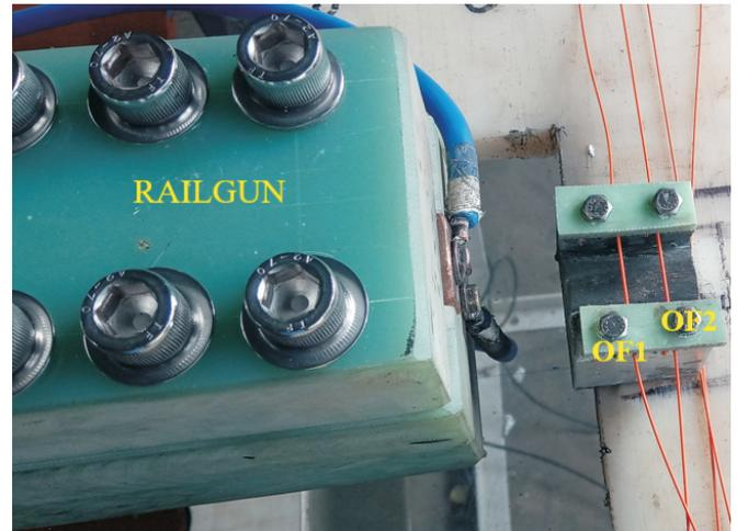
Fig.6: Muzzle velocity measurement setup.
