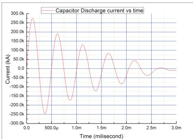
Fig.4: Capacitor discharge current with time.
