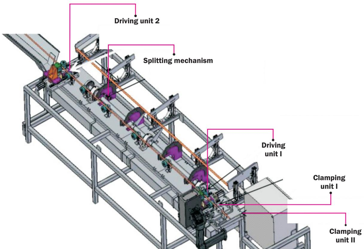
Fig.6: Pin welding automation system inside glove-box.
