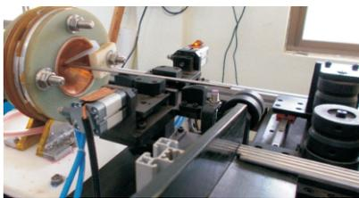
Magnetic Pulse Welding Setup
