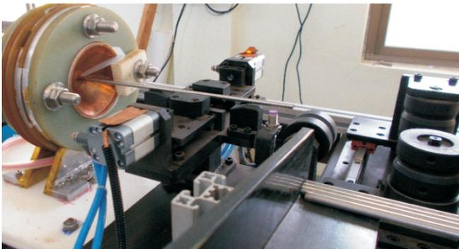
Fig.3: Magnetic pulse welding setup.
