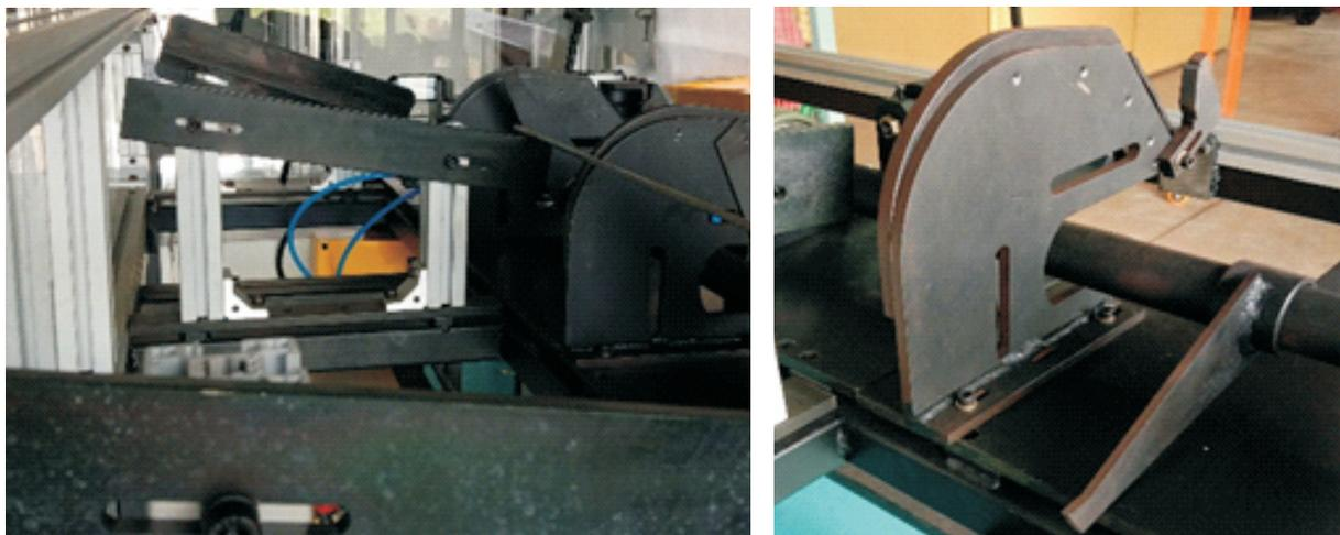
Fig.7: Inclined pin storage tray and pin splitting mechanism.
