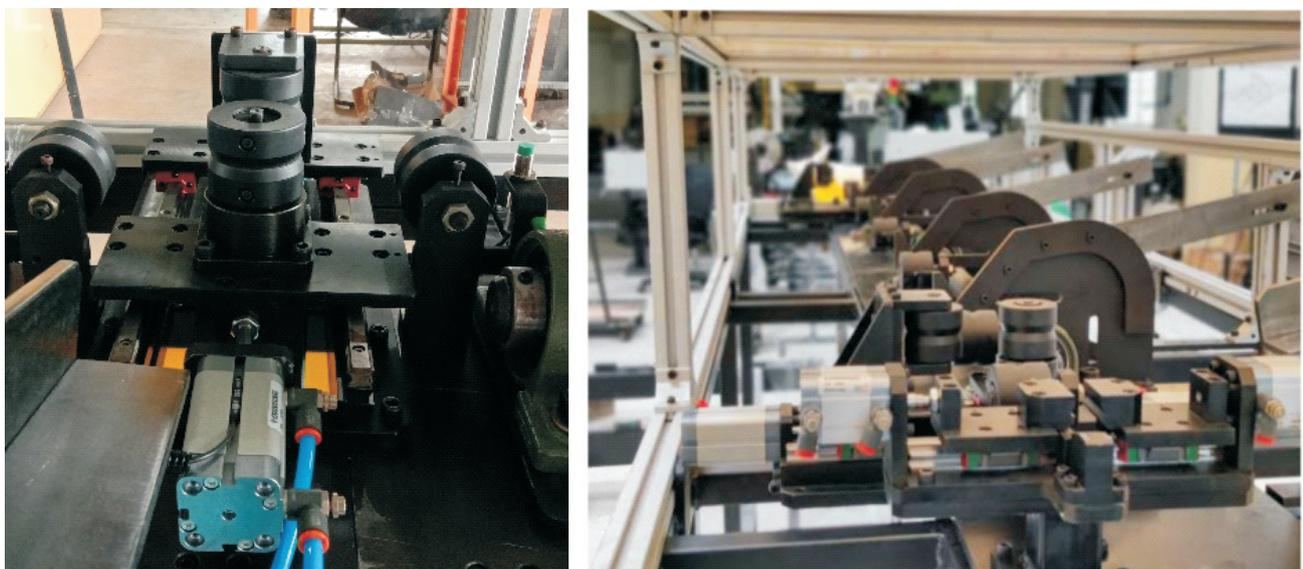
Fig.8: Driving rollers and supporting rollers.
