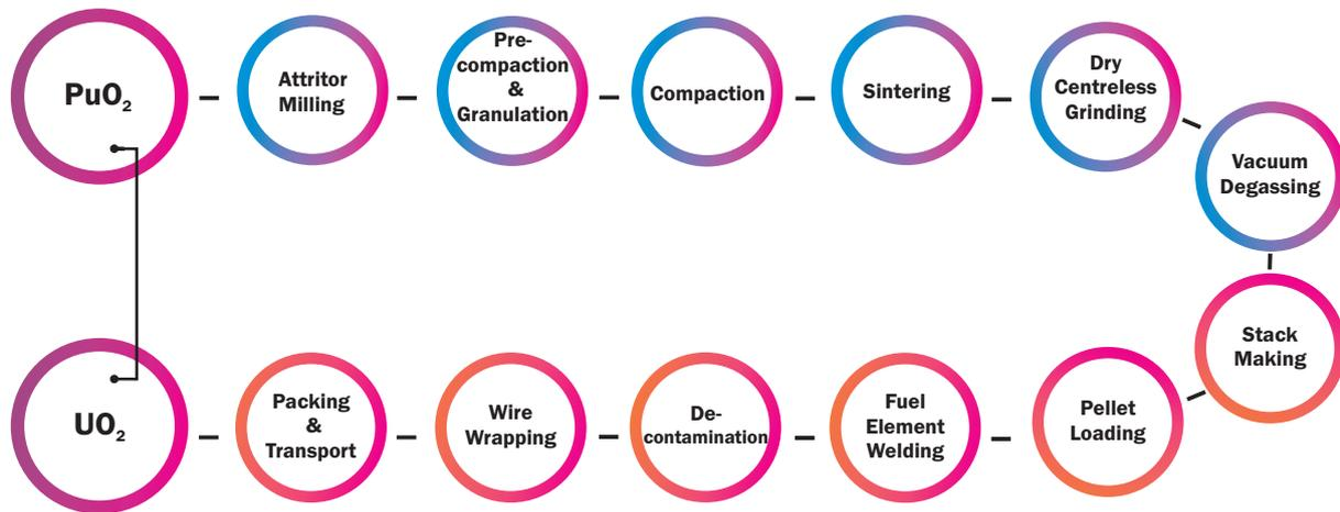
Fig.2: Flow chart of PFBR fuel pin fabrication.
