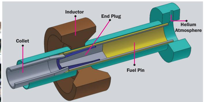
Fig.4: Section view of PFBR pin inside EM coil in helium atmosphere.
