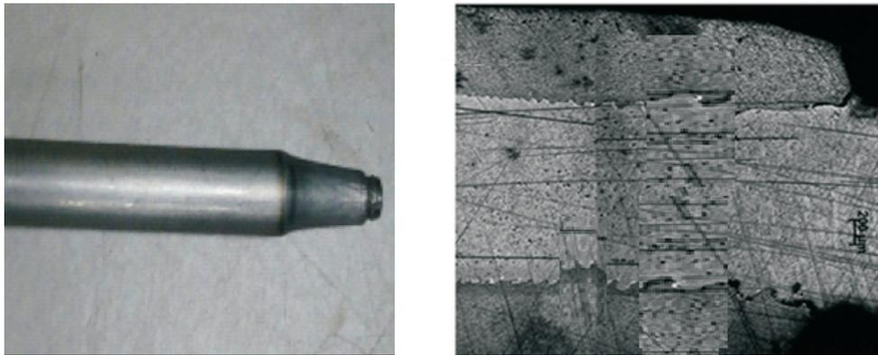
Fig.5: Welded fuel pin and microscopic image of weld interface.
