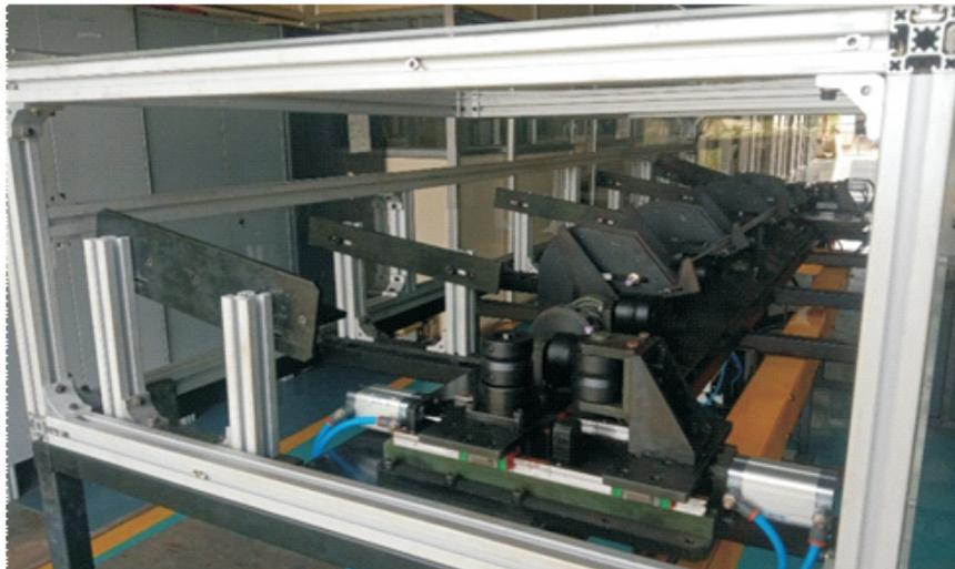
Fig.10: Driving roller second assembly and system with glove-box with exit bin.
