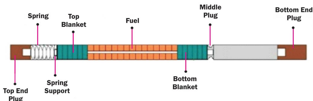
Fig.1: Schematic of PFBR fuel pin.
