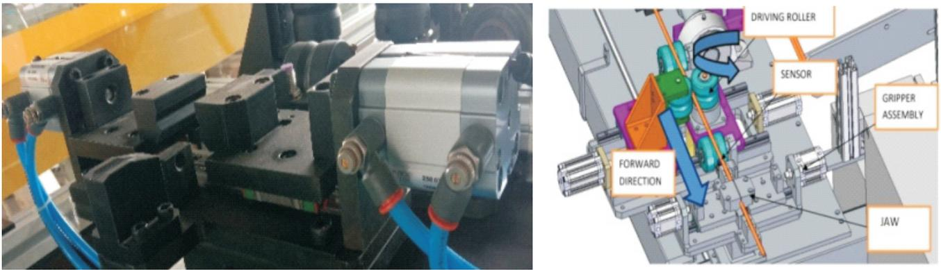
Fig.9: Gripper assembly and pin position during welding.
