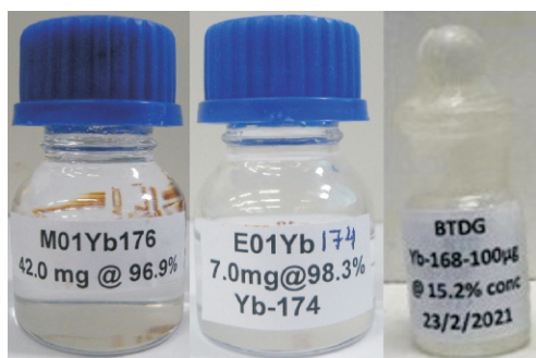
Fig.8: Sample product in liquid form recovered from enrichment experiments for Yb isotopes ^{176}\text{Yb} , ^{174}\text{Yb} and ^{168}\text{Yb} , respectively.
