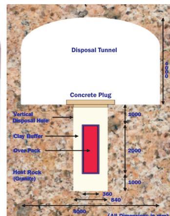
Fig.2: Schematic view of vertical disposal pit.
