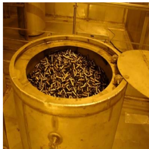
Hull Drum filled with hulls
