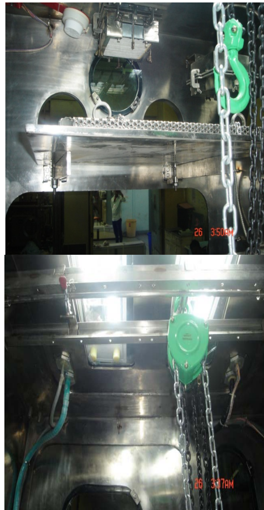
Figure 4: Roof lifting mechanism
