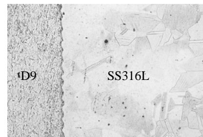
Fig. 10. (c) Optical micrograph indicating Characteristic waviness of EM weld sample at weld interface.
