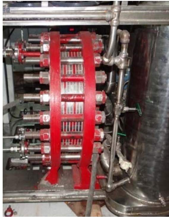
Fig.5 Six Cell module stack ( H_2 production capacity : 1.2 \text{ Nm}^3/\text{hr} )
