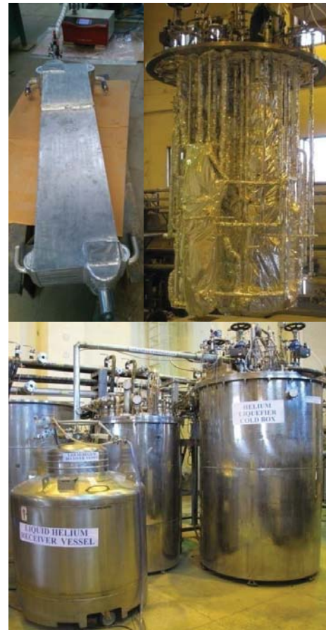
Figure 9: The PFHE, cold box piping and the developed cold box with the LHe receiver Dewar
