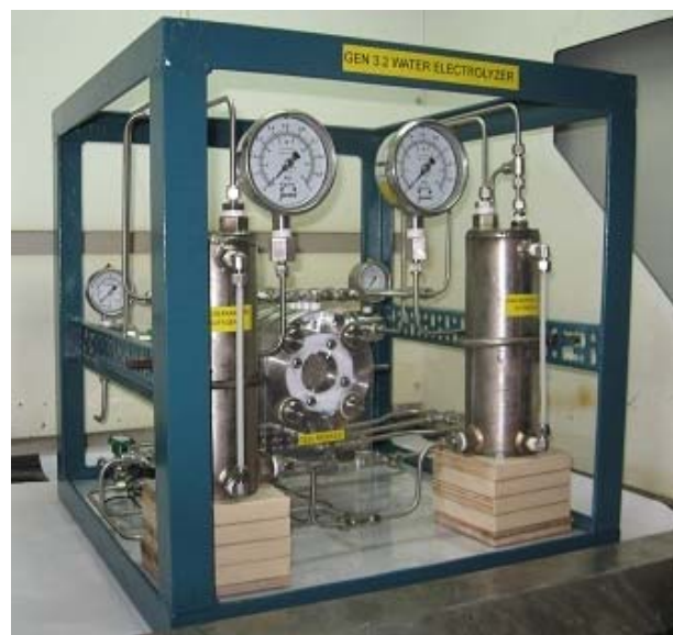
Fig.3 Bench scale electrolyzer unit (H 2 production capacity: 12 Nlph)
