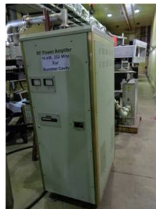
(a) 10 kW power amplifier and directional coupler
