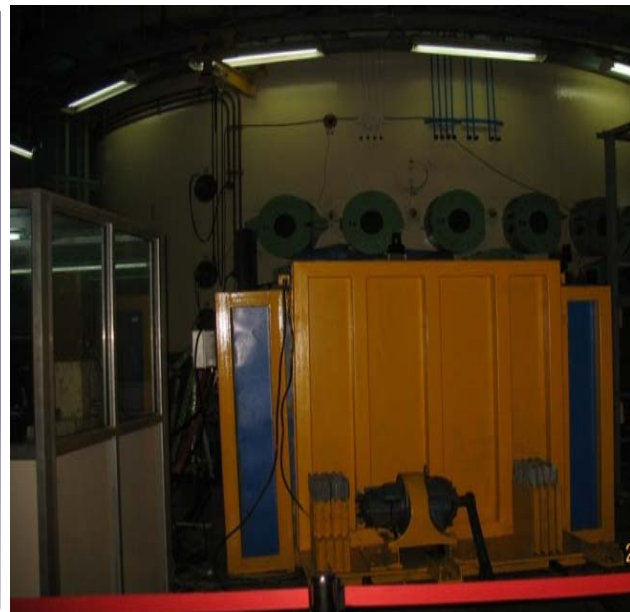
Figure 4 Schematic of Neutron collimator used in neutron tomography facility at CIRUS & Photograph of experimental facility
