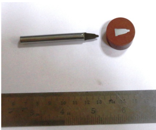
Fig. 11 Indicative sample of \Phi 6.6 OD \times 0.45mm thick \times 65mm long D9 steel to SS304 EMW sample. Casted sample was polished and etched with Oxalic acid.
