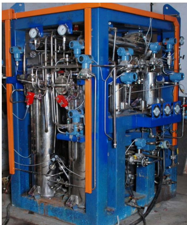
Fig.9 Alkaline water electrolyzer plant of 10 Nm 3 /hr Hydrogen production capacity
