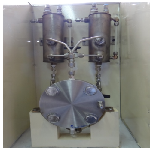
Fig.2 Lab scale electrolyzer unit (Hydrogen production capacity : 4 Nlph)
