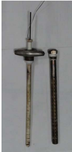
Fig. 4 In-house developed oxygen sensor
