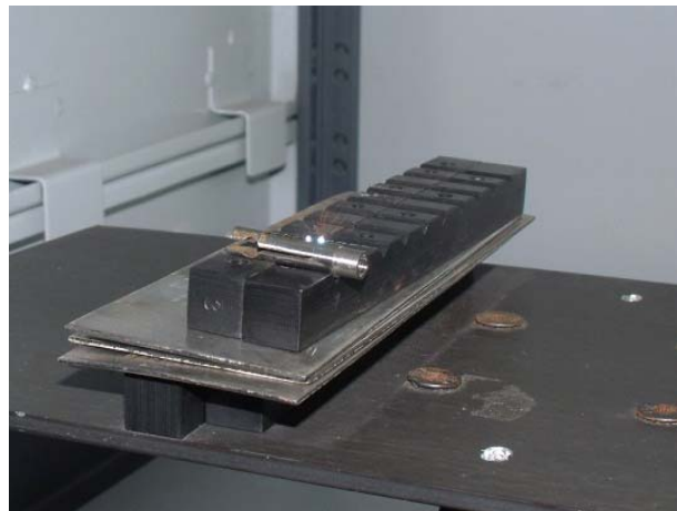
Figure 15: Laser marking using pulsed fiber laser
