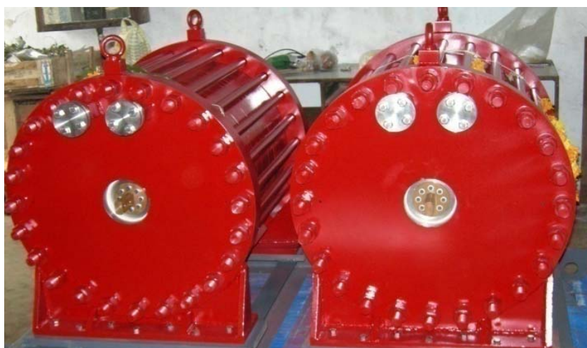
Fig.8 The cell module stacks with Hydrogen production capacity of 5 Nm 3 /hr each
