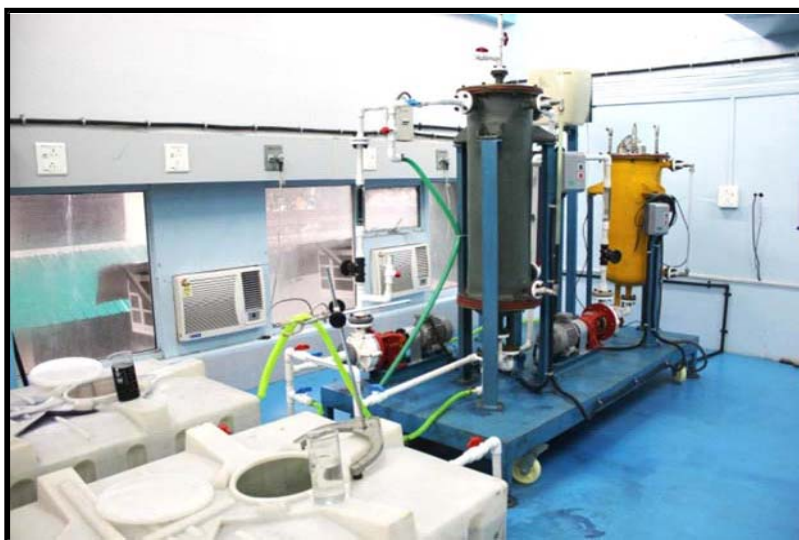
Figure 4. Radiation grafted cellulose based pilot plant waste water treatment setup
