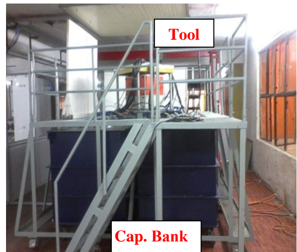
Fig. 8 (b) Photograph of 180 kJ energy storage capacitor bank and EM Tool
