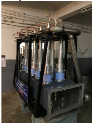
(c) 800 kW RF load @352 MHz
