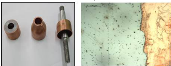
Fig. 9. Photograph of Sample of (a) Copper tube and soft iron disc (b) Optical micrograph of interface
