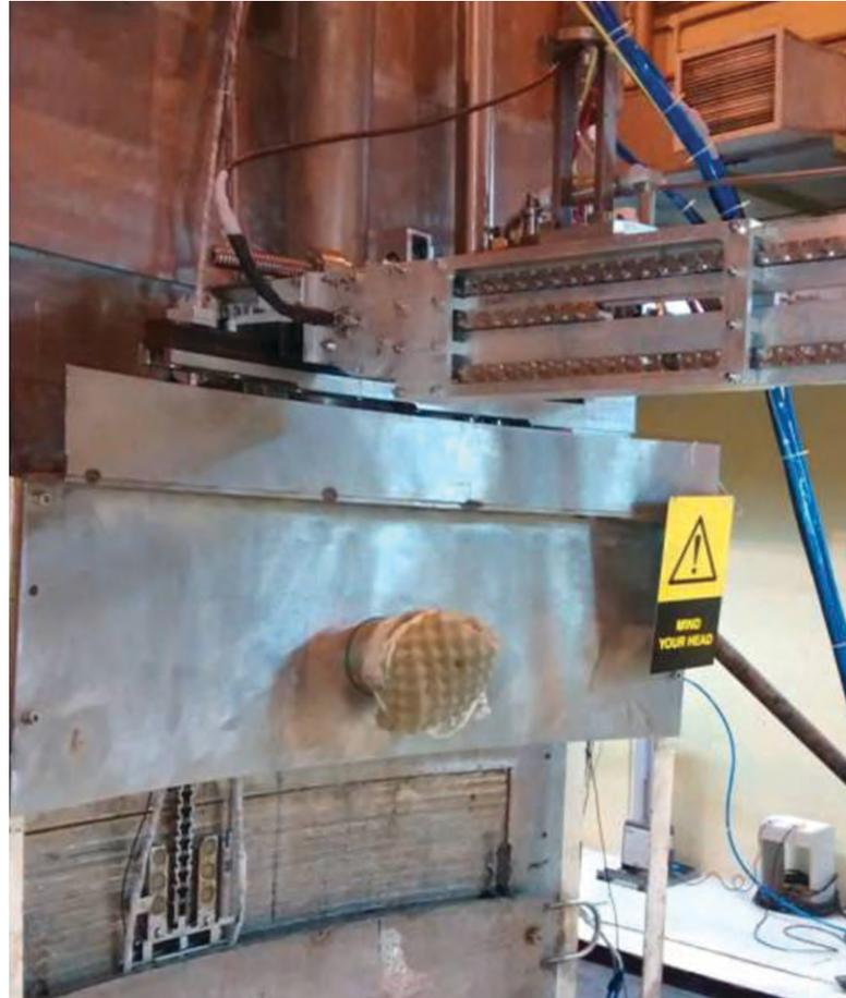
Fig. 15: Horizontal Probe holder entering in the annular gap of test set up
