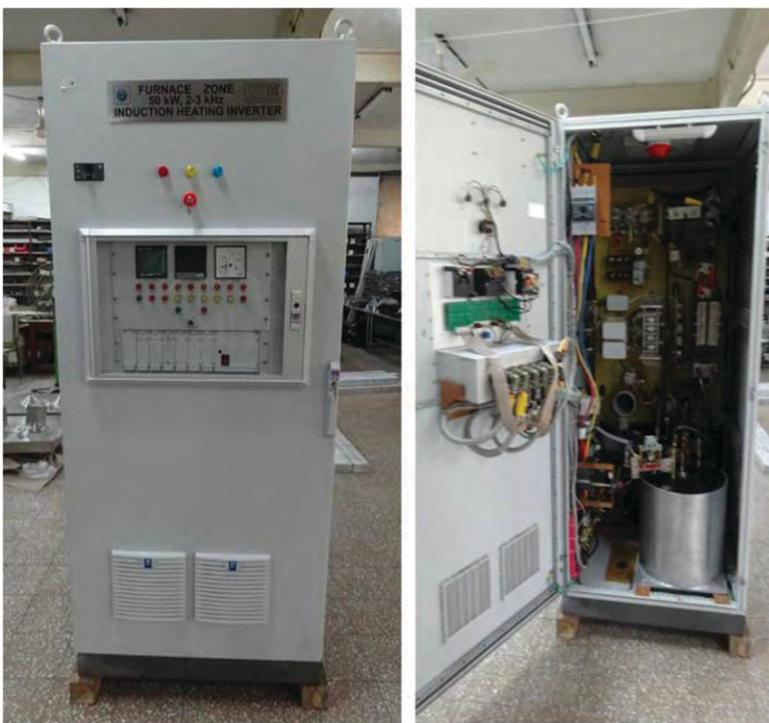
50kW Induction Heating Inverter
