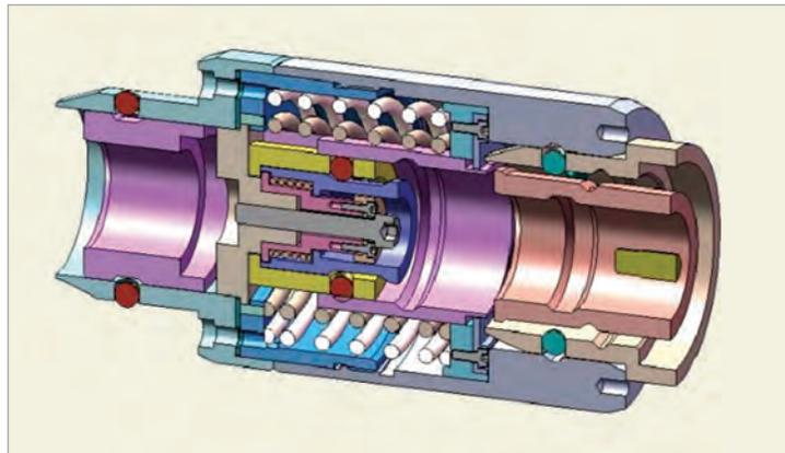
Fig. 4: SSP adaptor, 3D visualization of cross-section
