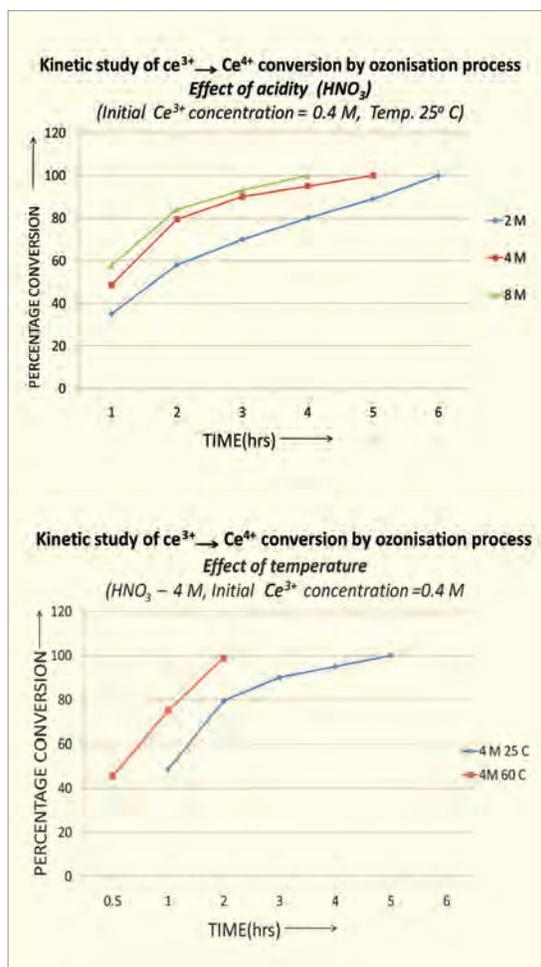
Fig. 2: Effect of acidity and temperature on Ce<sup>3+</sup> to Ce<sup>4+</sup> conversion by ozone
