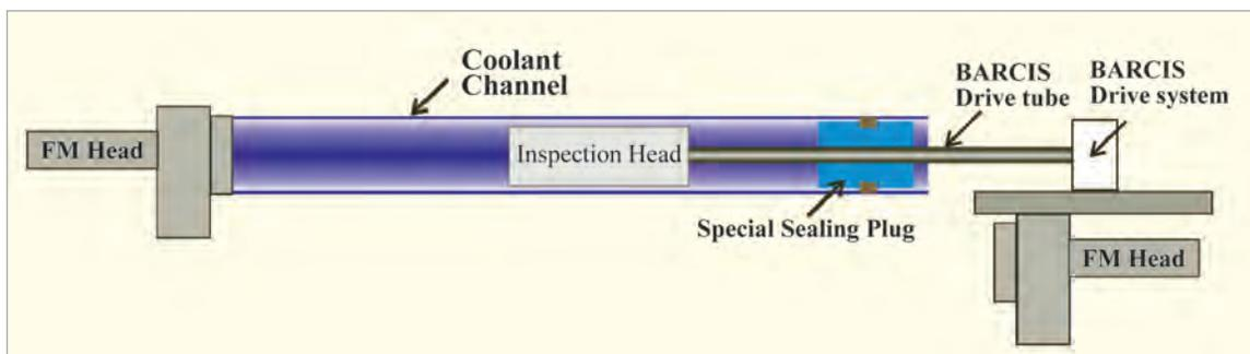
Fig. 1: BARCIS schematic during operation
