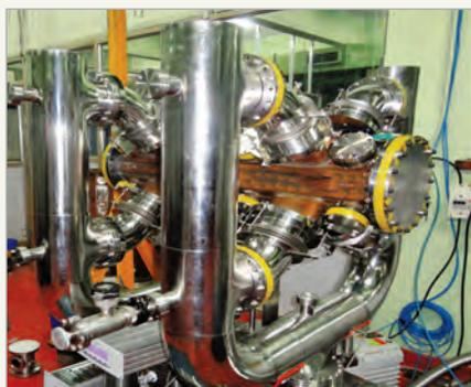
Fig. 1: 400 keV RFQ with its vacuum manifold. It has been tested for vacuum of  $4 \times 10^{-6}$  Torr
