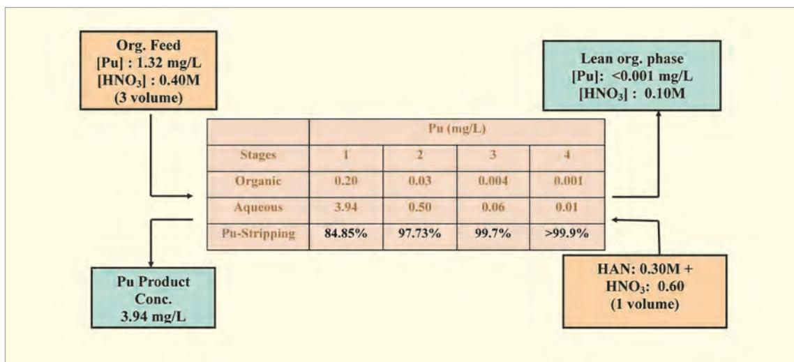
Fig. 7: Results from counter-current stripping run
