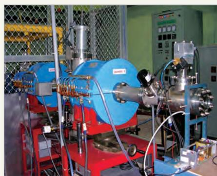
Fig. 4: LEBT test bench with solenoid magnets
