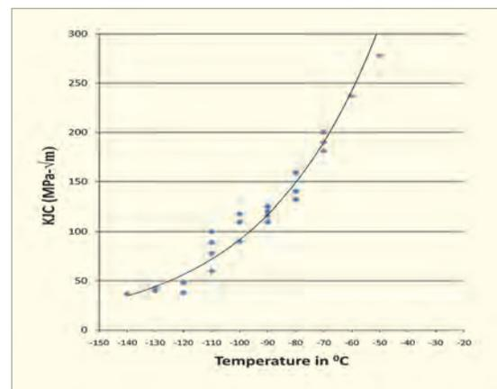
Fig.2: Scatter of fracture toughness data in transition range
