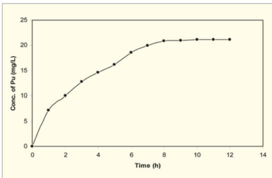
Fig. 5: Decontamination behaviour of alpha contaminated SS spatula
