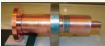
Fig. 2: 50 kW Co-axial RF Coupler.
