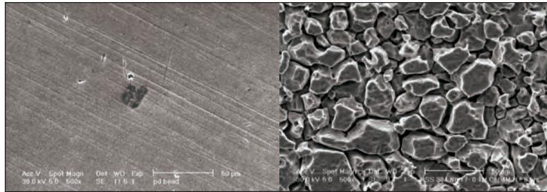
Fig. 3: Surface morphology of virgin and corroded SS planchet
