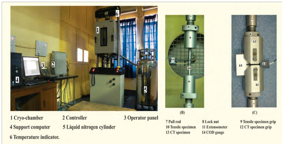
Fig.3: Photograph of 100 kN grip capacity Universal testing machine with low temperature test set up
