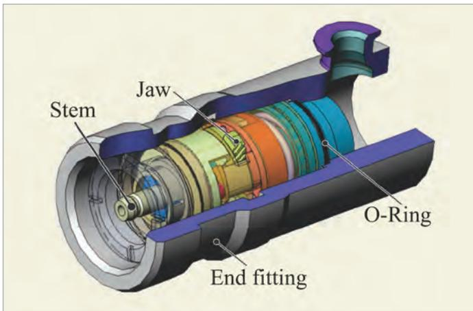
Fig. 2: 3D visualization of Special Sealing Plug installed in End fitting
