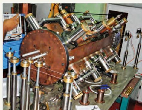
Fig. 3: The 400 keV RFQ with bead pull system
