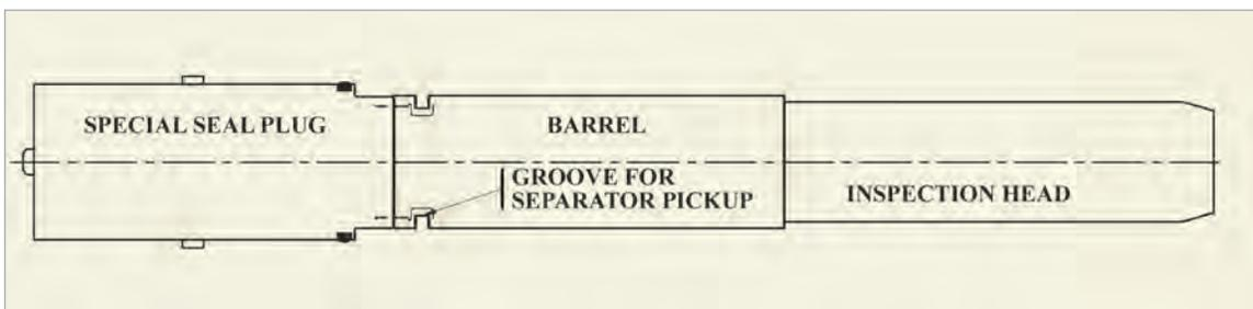
Fig. 3: Special Sealing Plug and Inspection Head assembly
