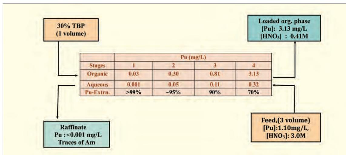
Fig. 6: The results from counter-current extraction run
