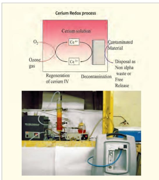
Fig. 1: Schematic of Cerium redox process and experimental setup
