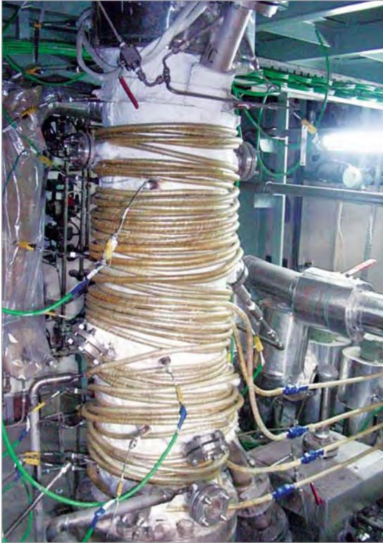
Fig. 3: 300 NB Denitration Column with induction heater coils
