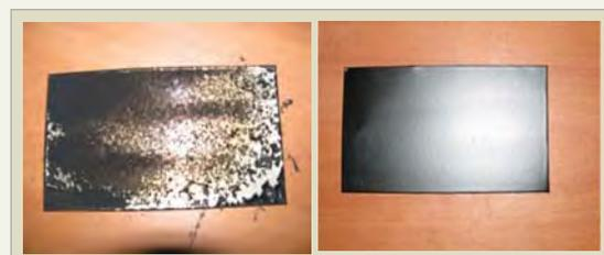
Plate with Coating (a) Before Curing (b) After Curing
