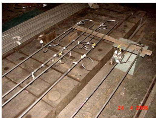
Fig. 6: U-tubes with tapings for Thermocouples and Impulse tube
