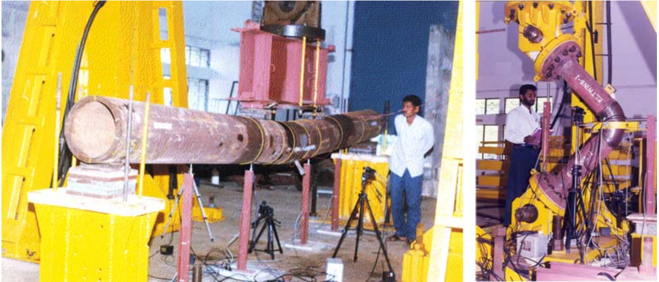
Fig.1: Photograph of pipe and elbow fracture test set-up
