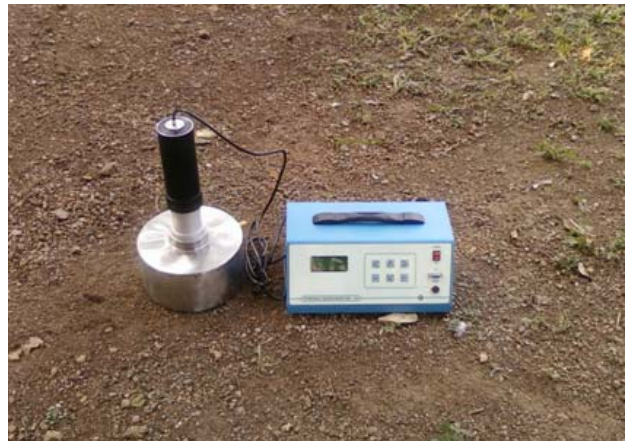
Fig. 6: Measurement of radon emission from soil using SRM
