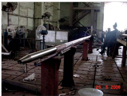
Fig. 9: SS Tube Plate End Of Fuel Rod Cluster
