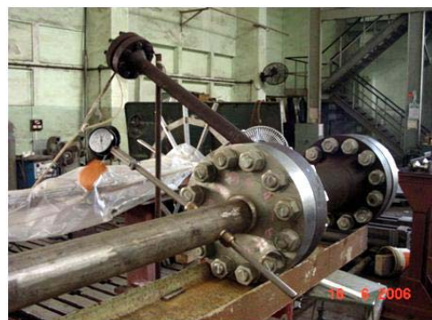
Fig. 11: FRCS Channel Assembly under Hydro-Testing
