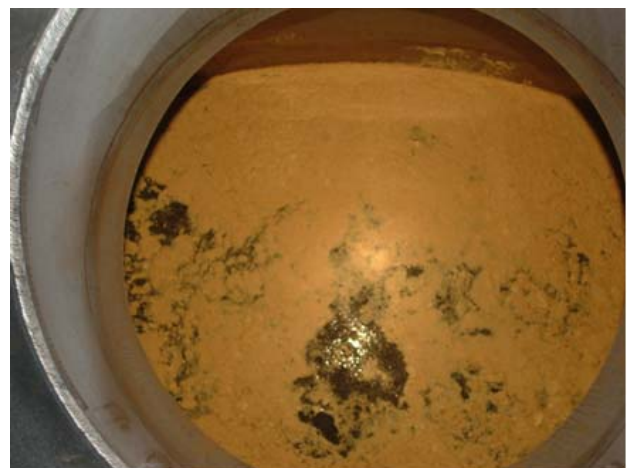
Fig. 2: Photograph of the organic mass separated during chemical precipitation
