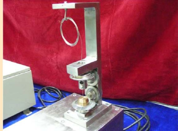
Fig. 3: Semi-automated welding system used for welding inside the hot-cell
