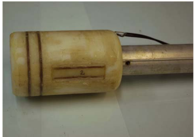
Fig. 3: Inspection Head containing garter spring coil and CT-PT gap coil
