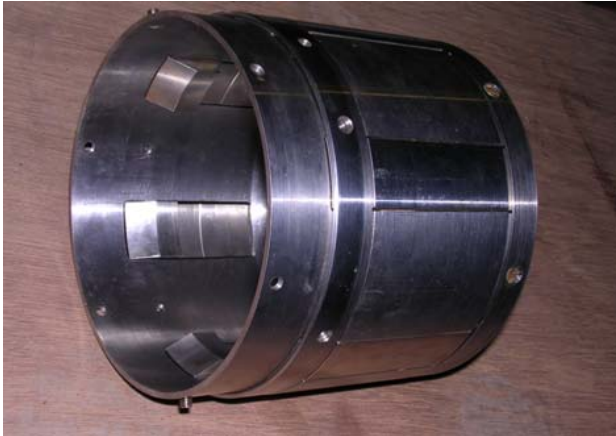
Fig 6 : End Fitting Blanking Assembly
