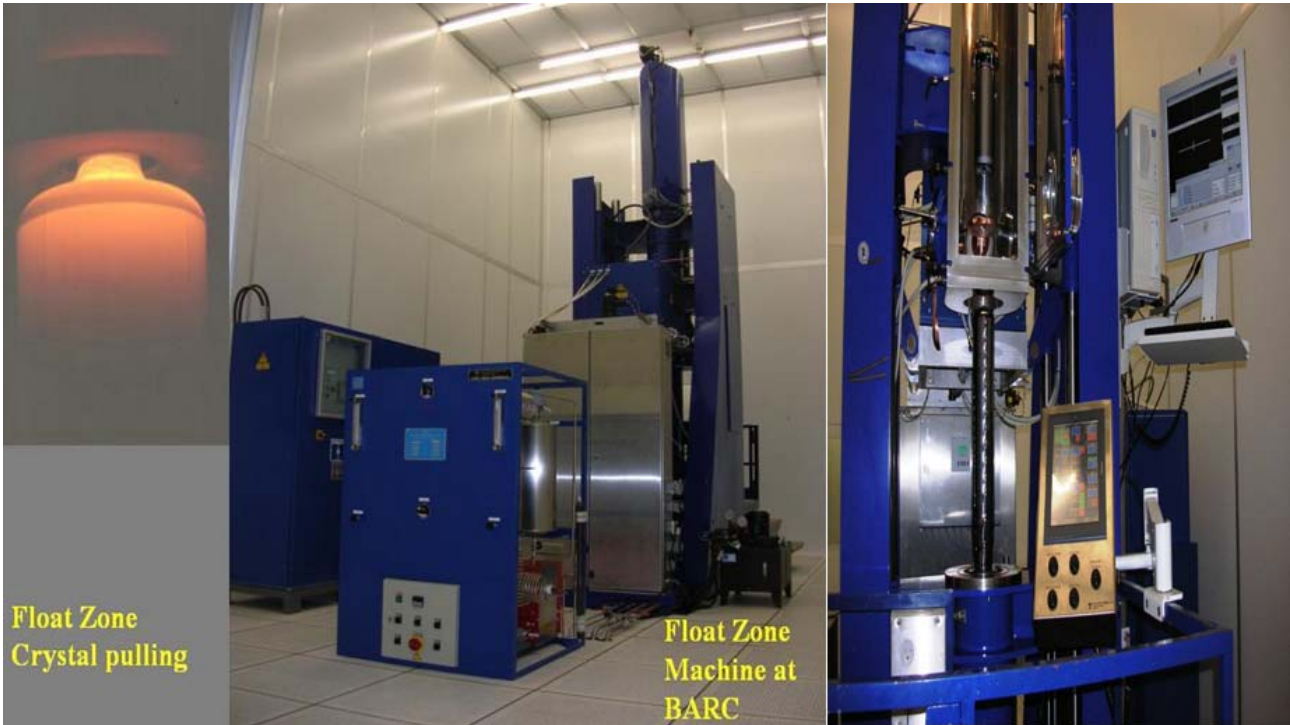
Fig. 6: FZ crystal pulling machine at BARC in class10 cleanroom & Grown Si crystal on machine
