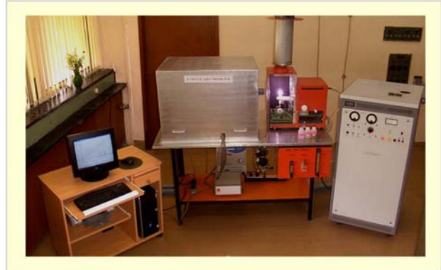
Fig. 13: Photograph of the analytical system using the echelle spectrograph
