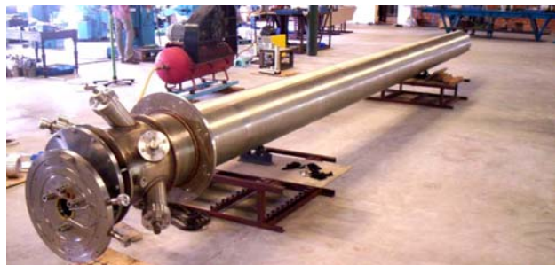
Fig. 15: Ten meter periscope under development for the PFBR Reactor
