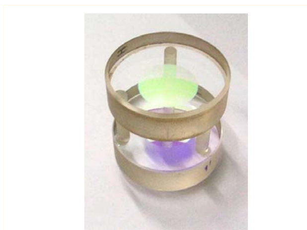
Fig. 9: Air spaced Fabry-Perot Etalon of free spectral range 7.5 GHz and aperture 25 mm
