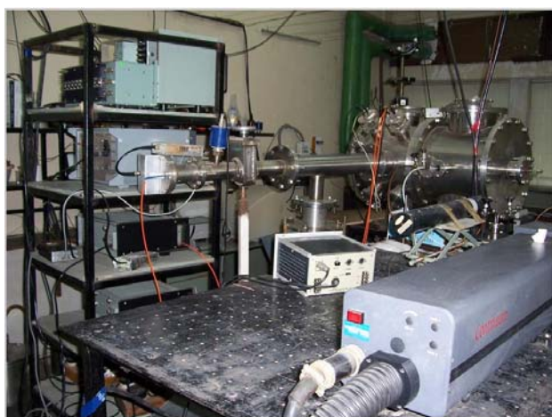
Fig. 1: Photograph of time-of-flight mass spectrometer indigenously designed and fabricated at Chemistry Division, BARC.
