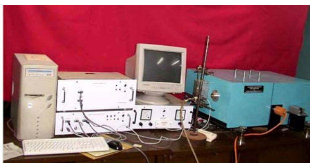
Fig. 7: Half meter spectrometer with data acquisition system
