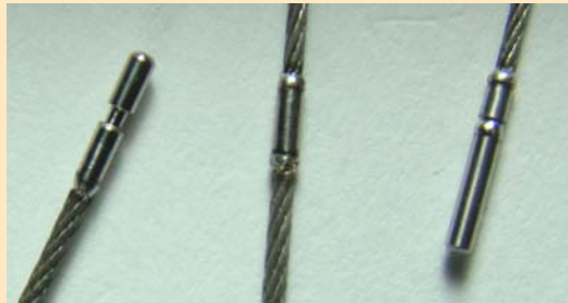
Fig. 2 (b): Welded Joints
