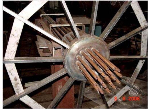
Fig. 10: Fuel Rod Cluster Ready for Insertion into the Channel
