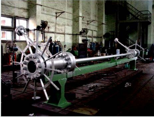
Fig. 12: Full FRCS Assembly ready for dispatch
