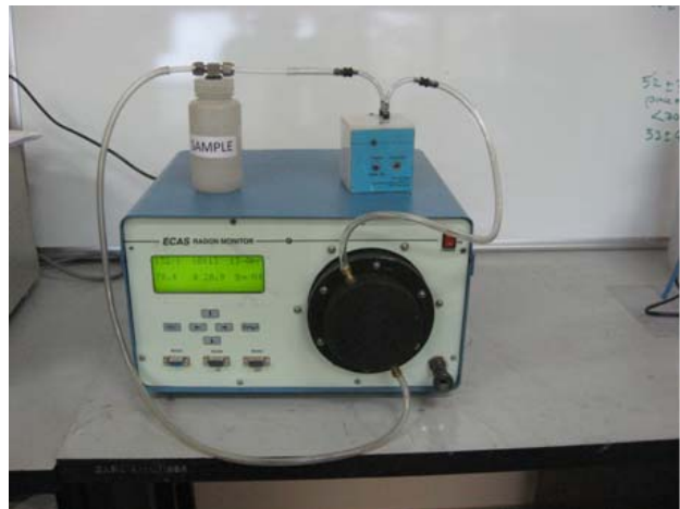
Fig. 7: Measurement of radon emission from a cement sample using ECAS
