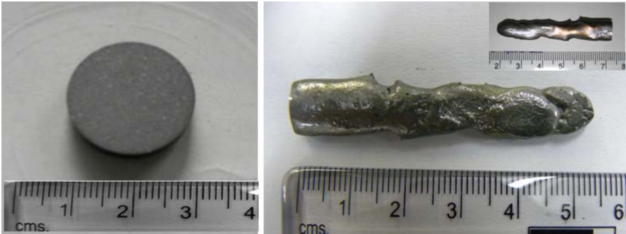
Fig. 2: Photographs of pellet of thorium powder (L) and thorium metal finger (R), produced by melting the thorium pellet in arc furnace
