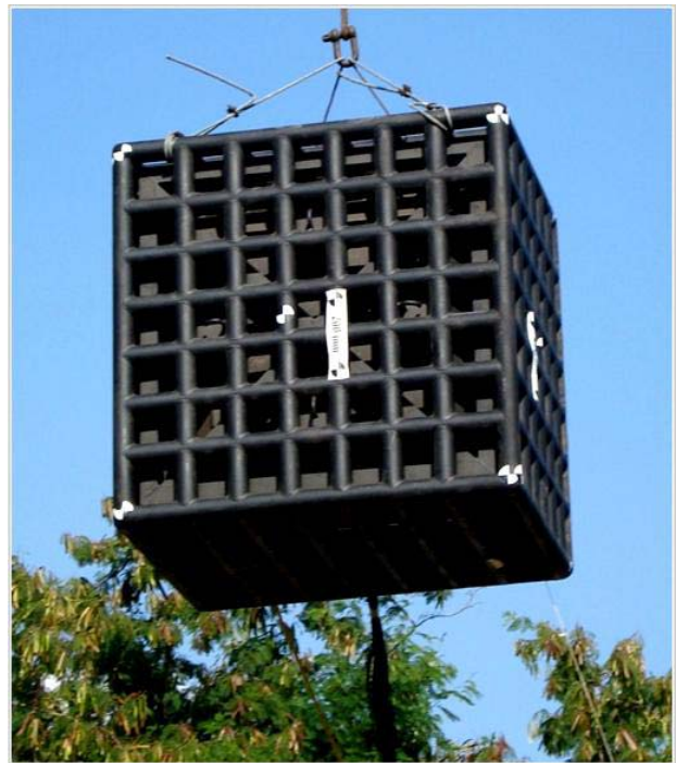
Fig. 3: Package before 9m free drop
