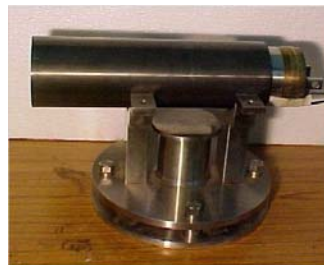
Fig. 3: IProMS tool head inside pressure tube.
