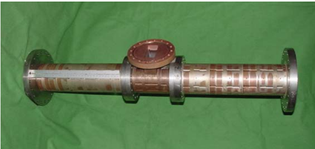
Fig.4: Brazen RF structure with 33 cells
