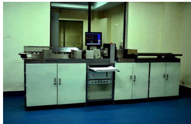
Fig. 1: Automated Eddy Current Test System for Testing of PRP Fuel
