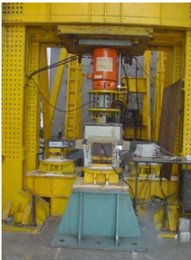
Fig.2: Photograph of Test Set-up and schematic of cruciform test specimen
