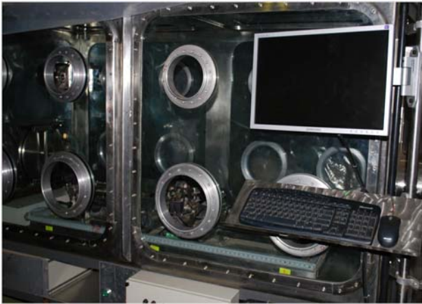
Fig. 2: Automated Fuel Inspection System for Testing of Metallic Fuel
