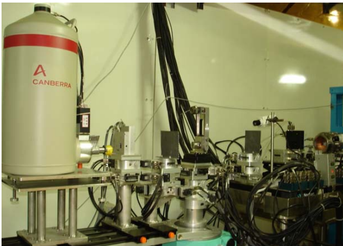
Fig. 2: EDXRD beamline installed at BL-11, Indus-2 (RRCAT, Indore)
