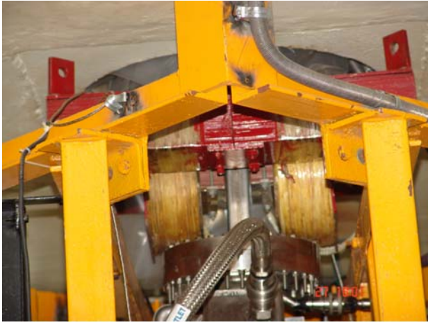
Fig. 7: Scan magnet mounted above horn
