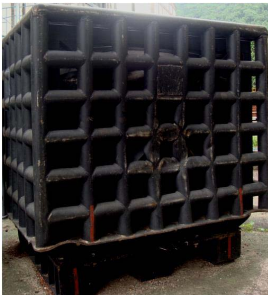
Fig. 4: Package after 9m drop and punch test
