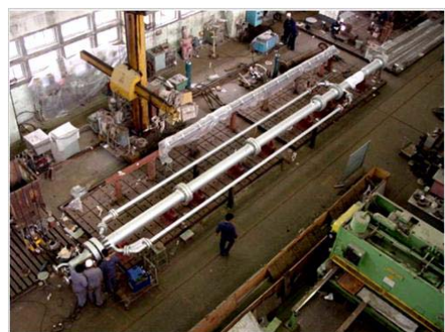
Fig. 7: Steam Generator final Assembly
