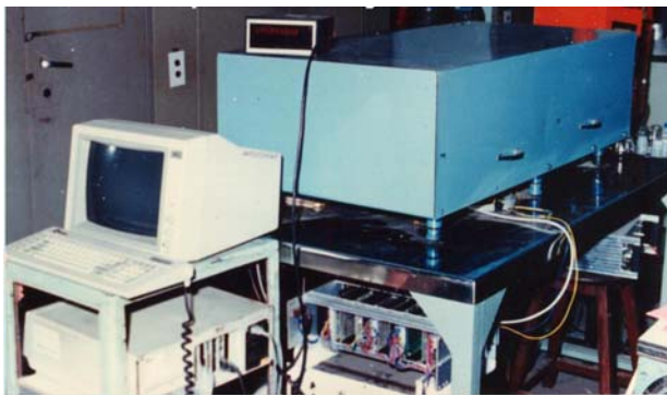
Fig. 3: One meter Czerny-Turner Scanning monochromator based sequential analysis system
