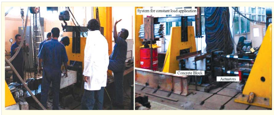
Fig. 7: Experimental Setup for the Tests at CTF (CDM, BARC)
