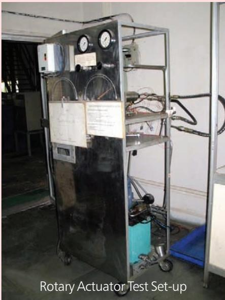
Rotary Actuator Test Set-up
