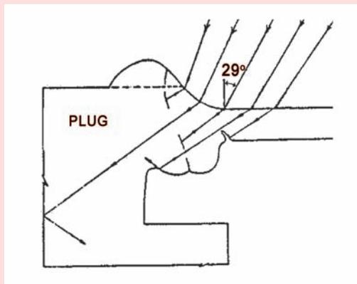
Fig. 5a: Ultrasonic testing of end cap welds for lack of fusion and root cracks.
