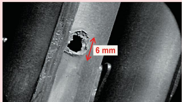
Fig. 19d: Another hole due to hydride blister is seen in the same fuel pin clad near middle bearing pad.
