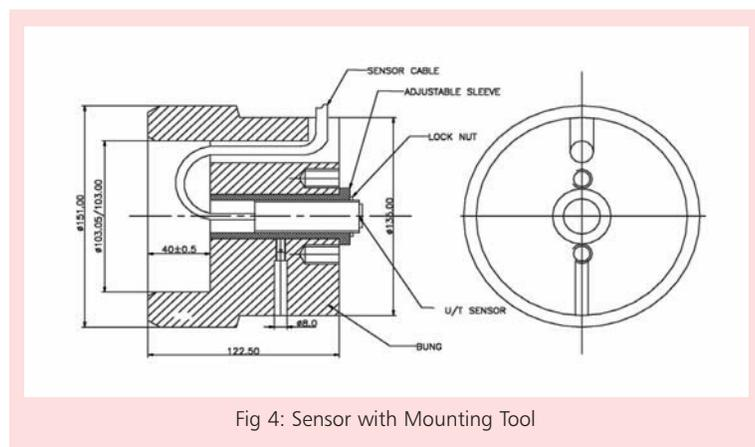
Fig 4: Sensor with Mounting Tool
