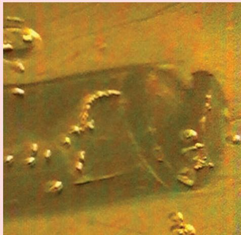
Fig. 4a: Nitrogen gas bubbles coming out of the leak in the end cap weld.
