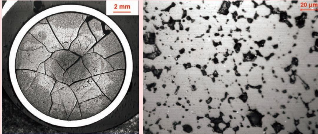
Fig. 15: Examination of metallographic samples of a pin from the AC-2 cluster revealed a central dark porous region as shown in the figure. The centre of the fuel revealed grain growth and interconnected pores at the grain boundaries as shown on the right. Such a microstructure is indicative of normal performance of a fuel.
