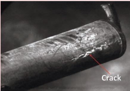
Fig. 3e : Crack on the cladding of an outer fuel pin from bundle no. 108305
