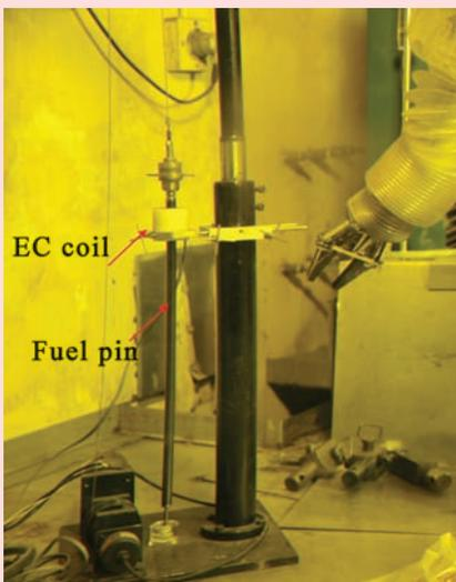
Fig. 7a Eddy current test set up.
