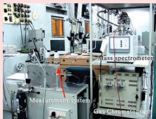
Fig. 8b The analysis part of the set up comprising of gas chromatograph and a quadrupole mass spectrometer.
