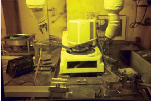
Fig. 9a: Metallographic preparation set up inside the hot cell.
