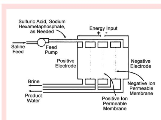
Fig.4: Electrodialysis setup
