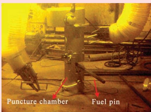
Fig. 8a :A low dead volume puncture chamber used for measurement of volume of released fission gases.
