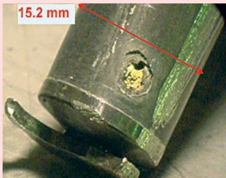
Fig. 19c: A pin-hole near the end plug weld of the fuel element. The  $UO_2$  had got oxidized by the steam generated due to ingress of water in the pin.
