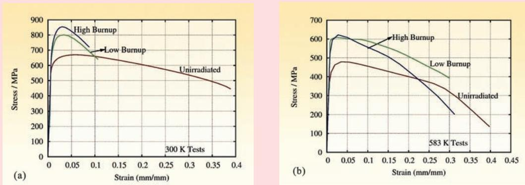
Fig. 11: Circumferential tensile deformation behaviour of low and high burnup fuel pin claddings, (a) at ambient temperature (300 K) showing irradiation hardening and reduction in clad ductility and (b) at 583 K showing significant increase in clad ductility at elevated temperature.
