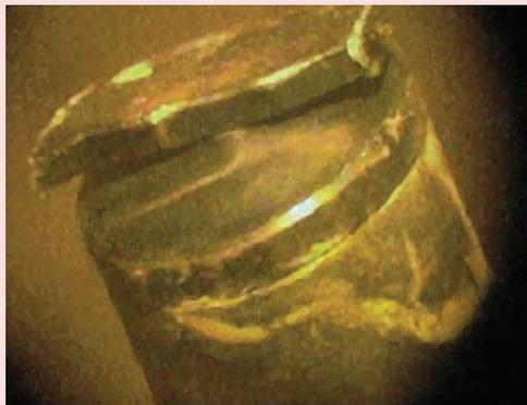
Fig. 4b: White patch around the zone containing leak near the weld.
