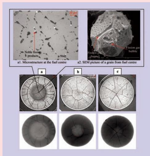
Fig. 17 Microstructure & β-γ autoradiographs of high burnup PHWR fuel
