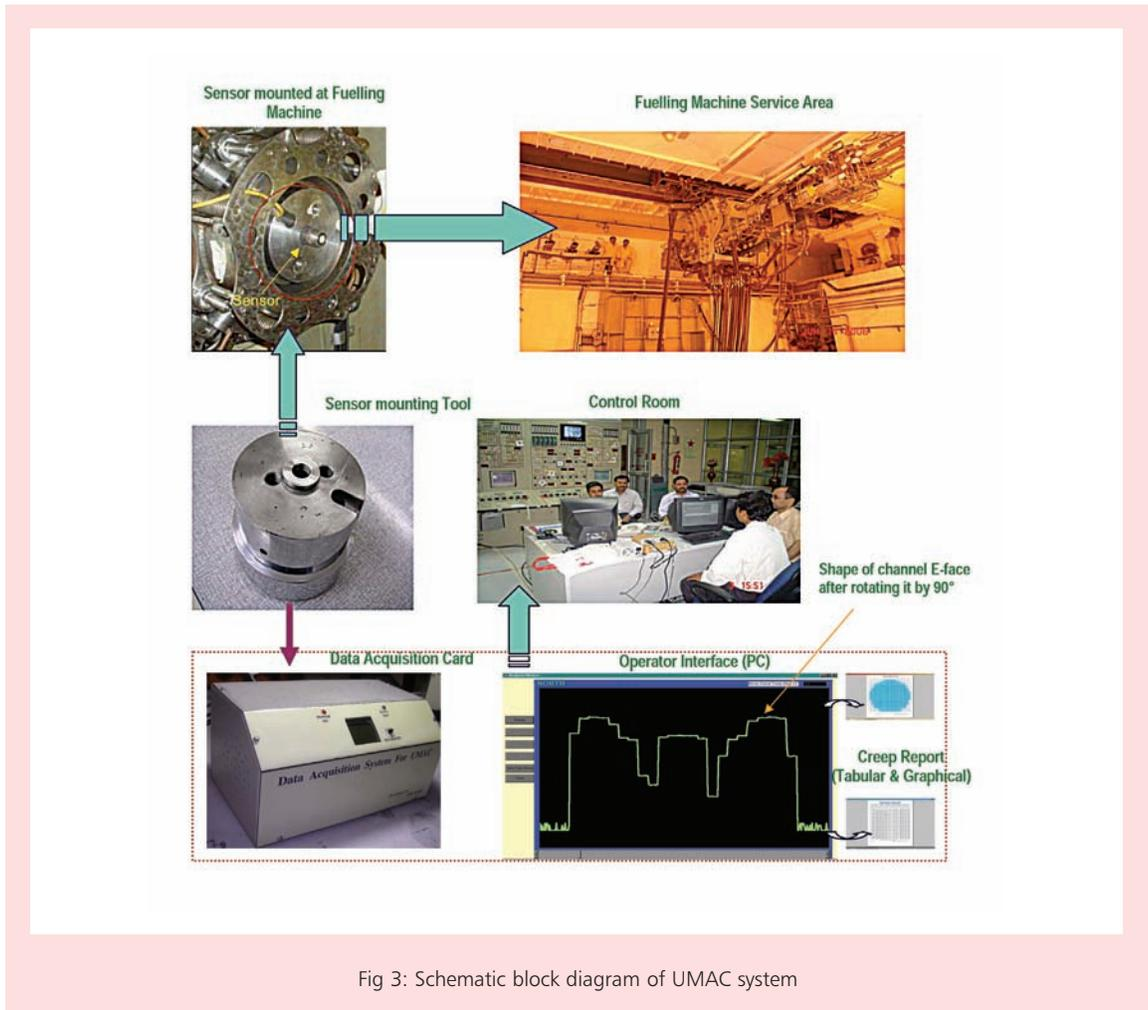
Fig 3: Schematic block diagram of UMAC system
