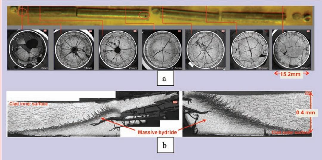
Fig. 19a: A fuel pin with a defective end plug weld operated in the reactor for a period of 710 days and accumulated a burnup of 4400 MWd/tU. Metallographic cross sections from different regions of the fuel pin are shown.
