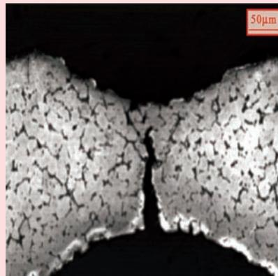
Fig. 13d Metallographic section through the failed region of the cladding. The grain boundary cavities indicate that the primary cause for failure is thermal creep.
