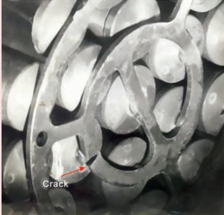
Fig. 3c: Cracked endplate of a PHWR fuel bundle.
