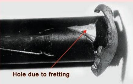
Fig. 3f: Fretting failures seen during the early stages reactor operation
