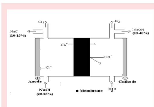
Fig.5: Schematic representation of chlor alkali electrolyzer.
