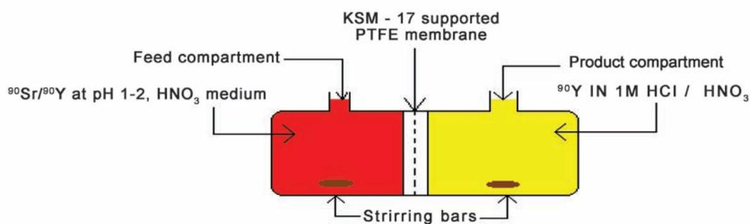
Fig. 1: Single Stage SLM Generator
