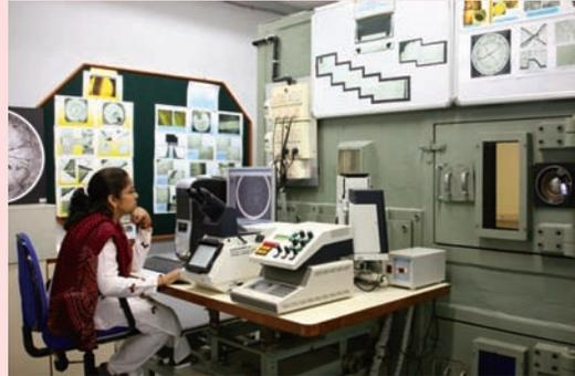
Fig. 9b: Remotised- shielded metallograph with radiation resistant optics used to examine samples from irradiated fuels
