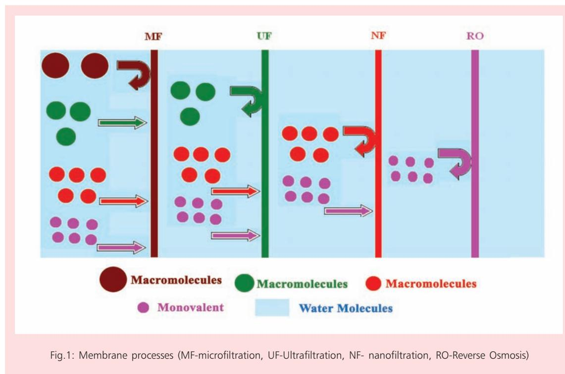
Fig.1: Membrane processes (MF-microfiltration, UF-Ultrafiltration, NF- nanofiltration, RO-Reverse Osmosis)
