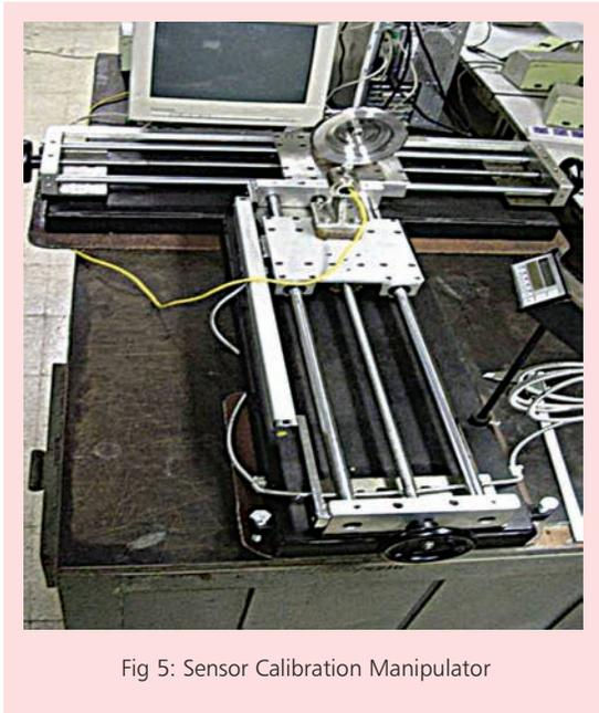
Fig 5: Sensor Calibration Manipulator
