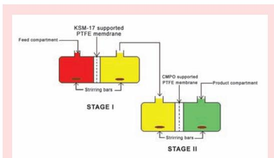
Fig. 4: Two stage Membrane Cell operated in sequential mode
