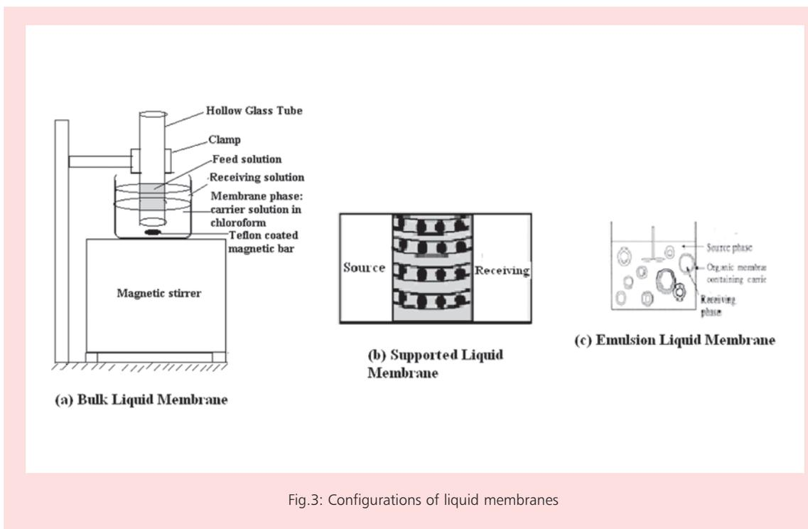
Fig.3: Configurations of liquid membranes
