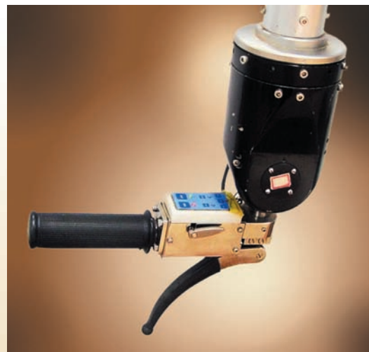
Fig. 5: Wrist and Handgrip of the Master Arm
