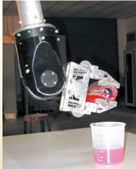
Fig. 15: ASM handling a glass flask. ASM can handle objects weighing upto 25 kg. It can also handle delicate object safely, using force control and force limit
