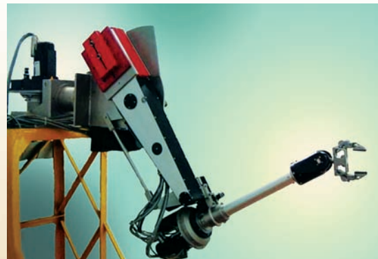
Fig. 3: Slave Arm in "Elbow-Down" configuration
