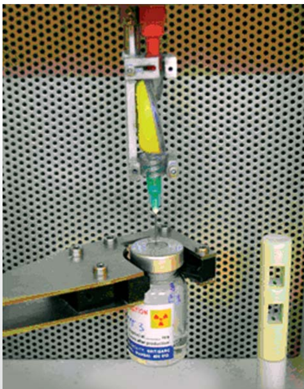
Fig. 2 : Dispensing unit: Vials getting dispensed through 0.2\mu filter one after another in a Class-100 area
