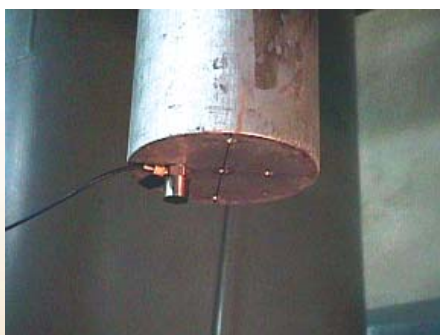
Fig. 9: Accelerometer attached to the bottom side of the guide tube
