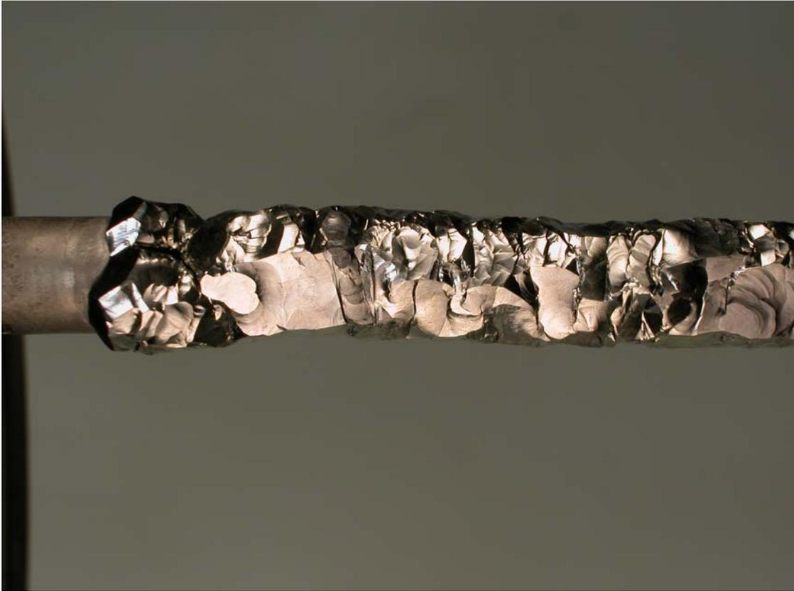
*Fig.4 Macrostructure of a section of crystal bar zirconium*
