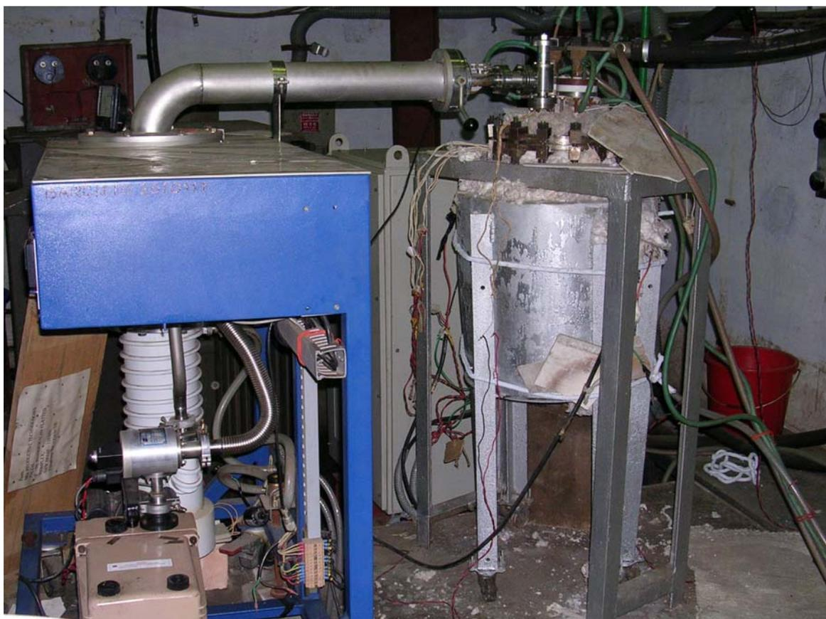
Fig. 2 Refining assembly with vacuum system and water cooled flexible copper cables
