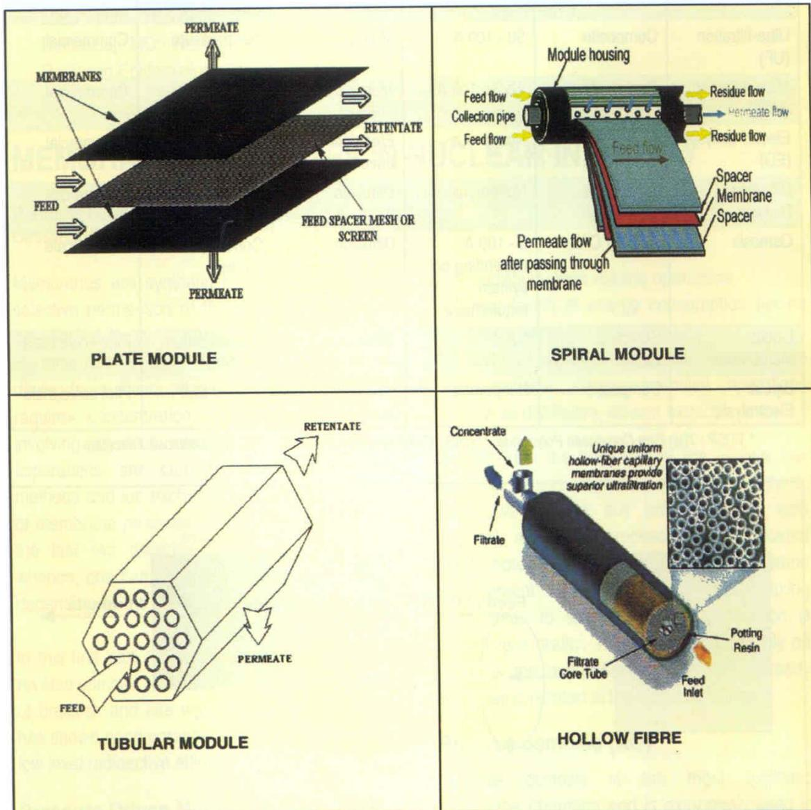
Fig. 2: Different configurations of Reverse Osmosis modules
