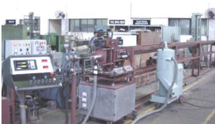
Remote cutting machine for guide sleeve
