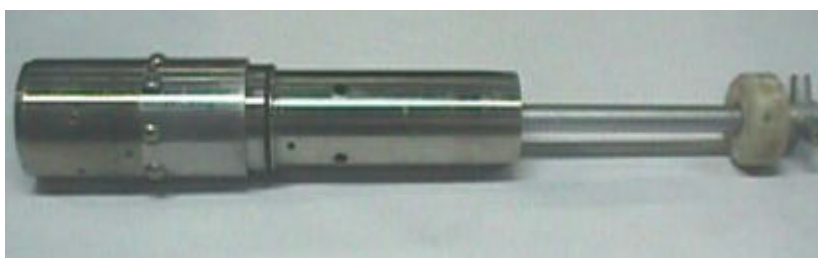
3 point micrometer for ID measurement of pressure tube
