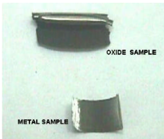
Sliver sample taken by WEST from pressure tube
