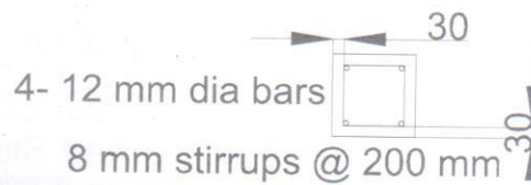
Figure 4 : Cross section details of column
