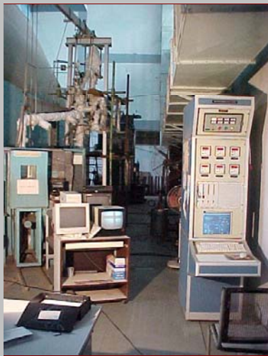
Facility at Apsara Reactor for Flow Pattern Transition Studies by Neutron Radiography
