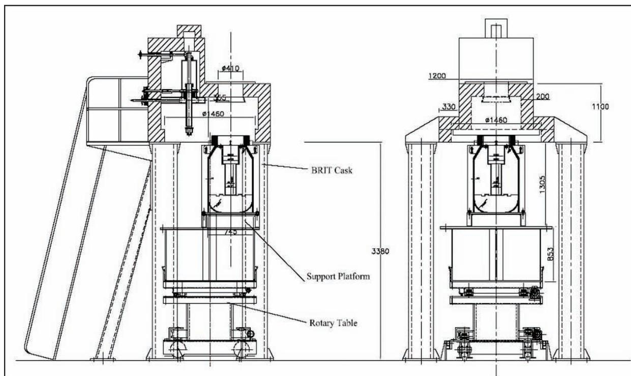
Fig. 8: Schematic of Cask Support Platform & Loading Station
