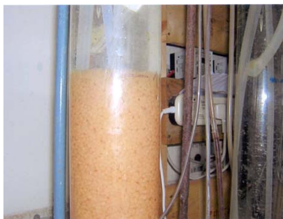
Fig. 2 Close up of a laboratory sequencing batch reactor (SBR) with cultivated aerobic granules
