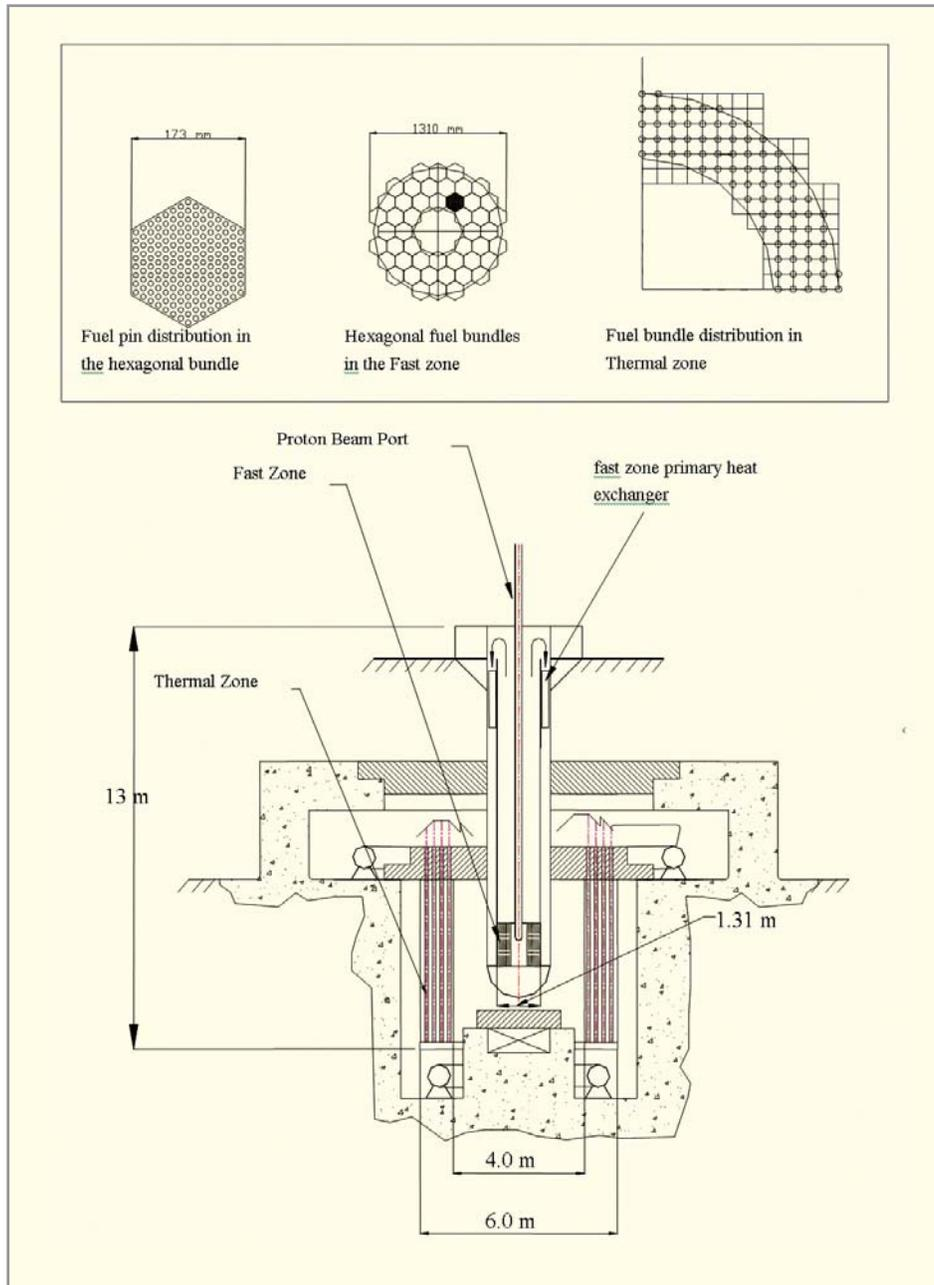
Schematic of fast-thermal ADS
