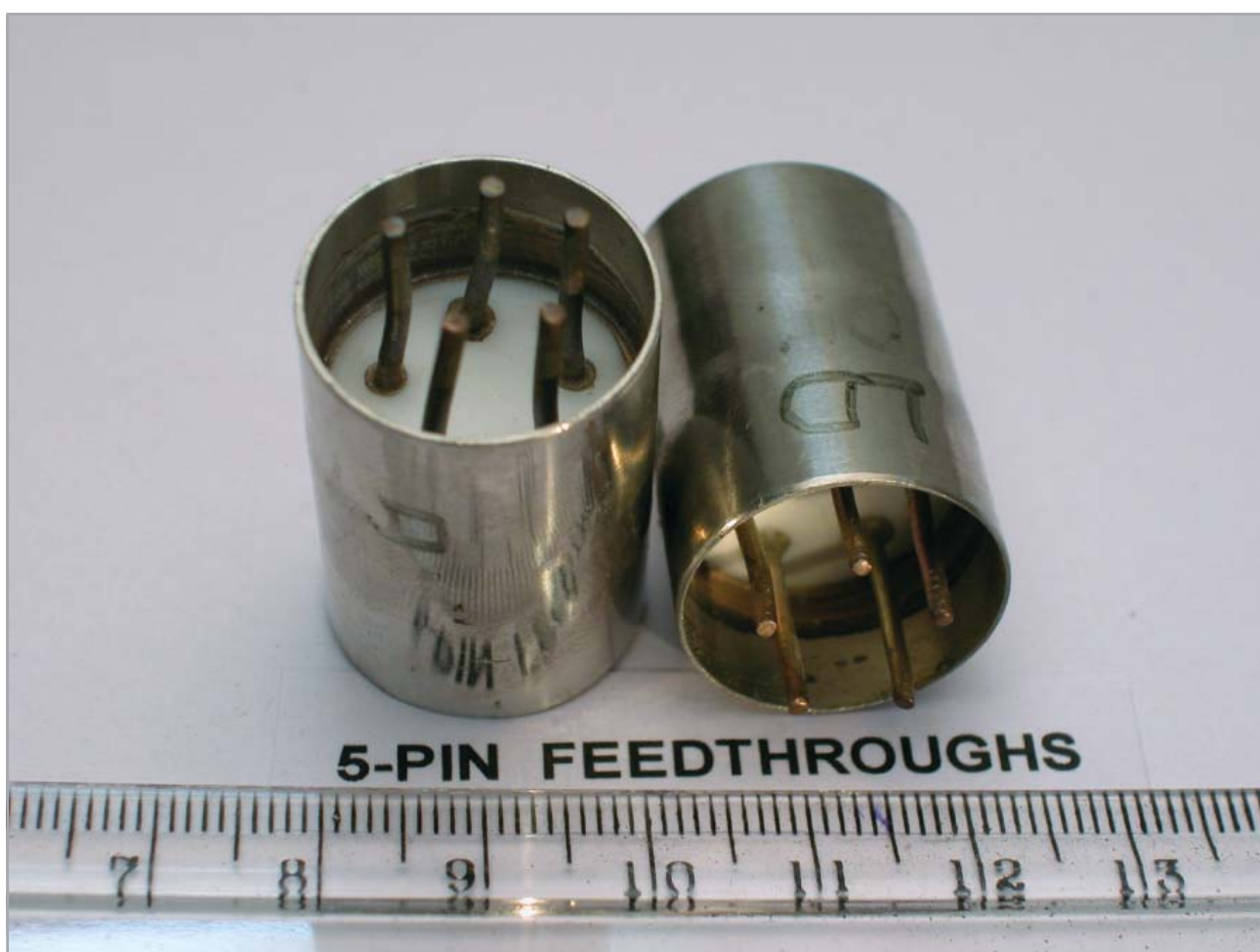
Indigenously developed 5-pin ceramic feed-throughs
