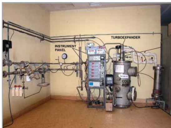
Laboratory test set-up built to test the performance of turboexpanders, efficacy of vacuum system, cryogenic insulation, indigenous temperature sensors and overall system performance and reliability
