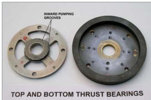
Top (L) and bottom (R) thrust bearings showing inward pumping grooves
