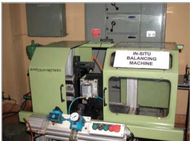
Balancing machine developed in conjunction with Shenck Avery for vertical in-situ balancing of rotors
