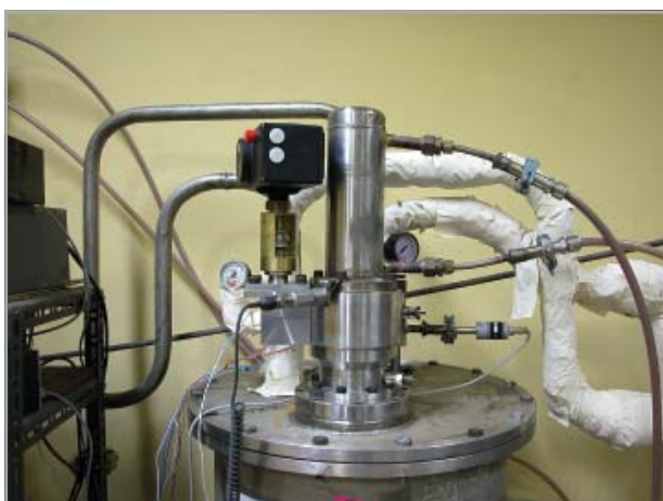
Turboexpander mounted on the test bench
