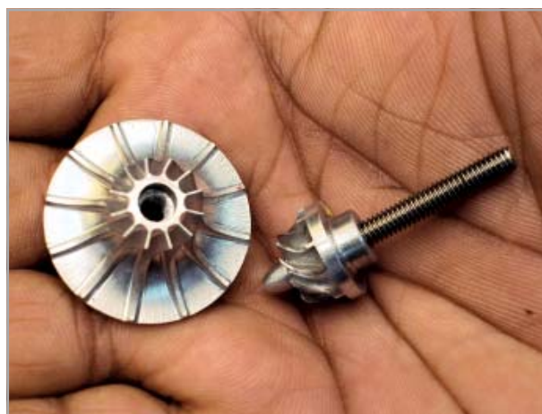
Miniature turbomachinery: expansion turbine and brake wheel
