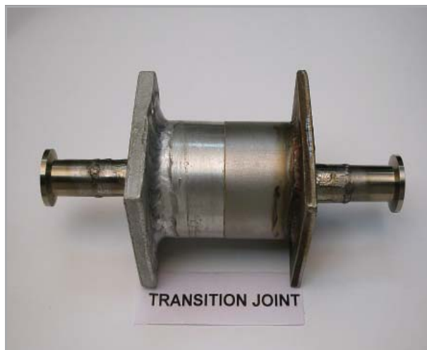
Transition joint between aluminium and stainless steel pipes
