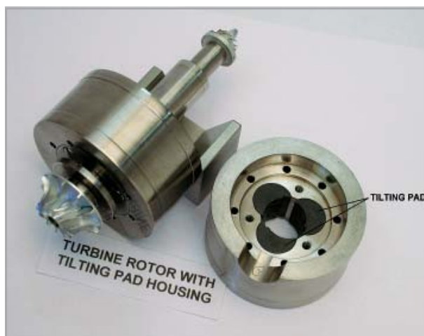
Turboexpander rotor with tilting pad bearing housing
