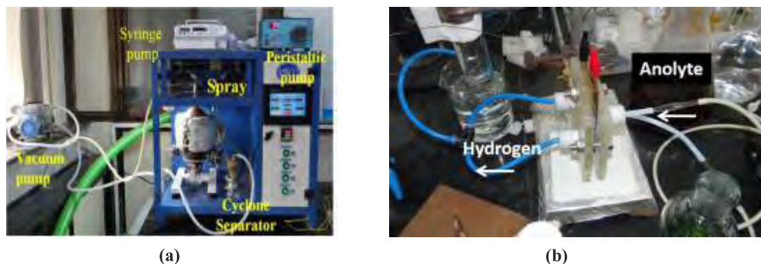
Fig. 2: Indigenously developed (a) spray reactor for CuCl_2 hydrolysis and (b) CuCl/HCl single cell electrolyser with Pt/C electrocatalyst based membrane electrode assembly (MEA)
