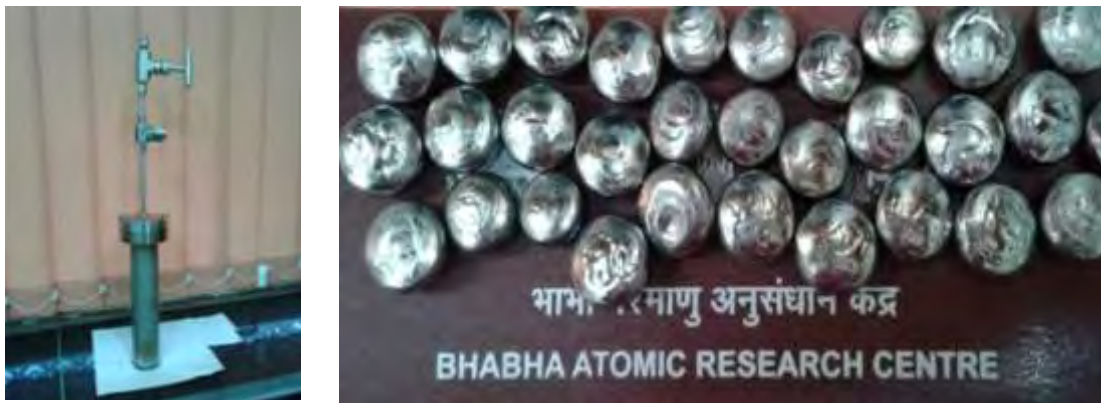
Fig. 3: Material developed for online hydrogen storage facility
