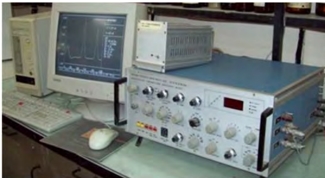
Fig. 1: The in-house developed computer controlled electrochemical system equipped with linear and pulse voltametric techniques
