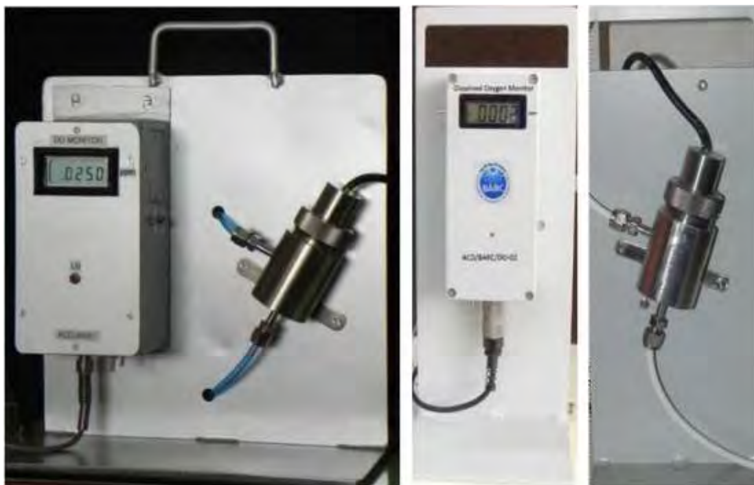
Fig. 2: Photograph of the dissolved oxygen monitor which has been developed and technology has been transferred to several companies, Technology code: CH32ACD, Website, http://barc.gov.in/technologies/dom1/index.html
