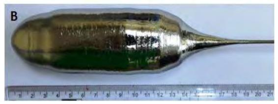
Fig. 7: (A) ~8 to 9N pure germanium ingot from Zone-refining unit, and (B) Single Crystal (<100>) of germanium (950 g) grown by TPD from ~8N pure germanium supplied by Chemistry Division.
