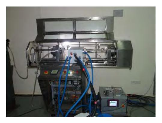
Fig. 6: Zone refining (ZR) unit with induction heating designed and fabricated indigenously in 2012.
