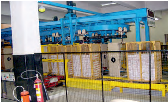
Figure 6: Product conveyor system in KRUSHAK Irradiator, Lasalgaon
