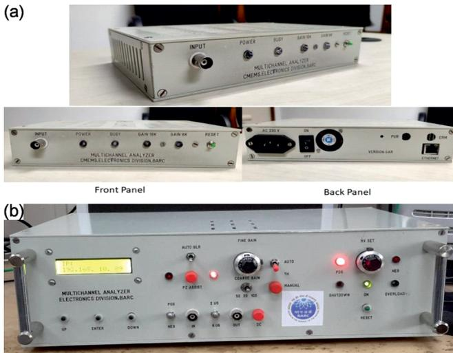
Fig.19: (a) 16k portable MCA module and (b) Integrated Multi-channel Analyzer (IMCA).
