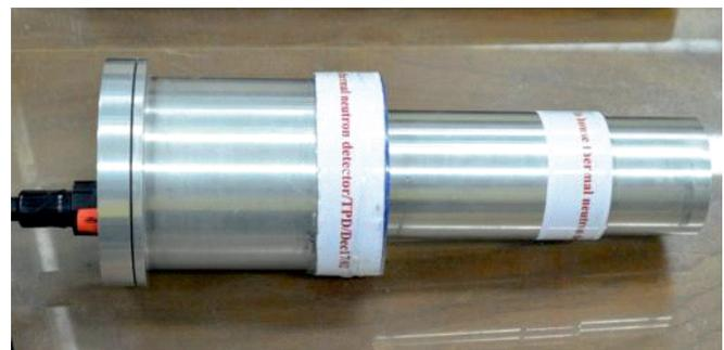
Fig.10: A USB based handheld thermal neutron detector employing Lil:Eu<sup>2+</sup> single crystal.
