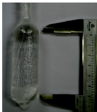
Fig.1: Single crystal ingot of YAP:Ce.
