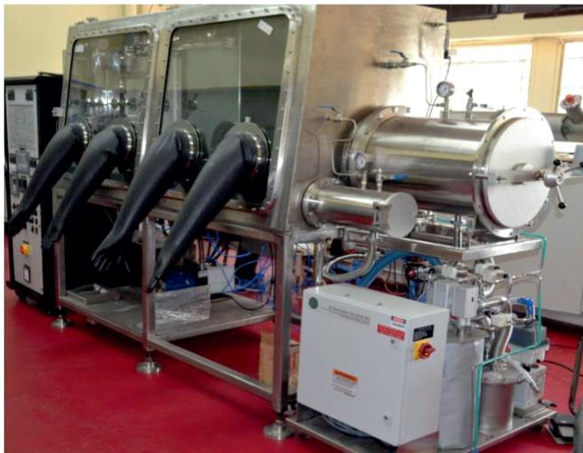
Fig.9: Glove box equipped with thermal evaporation system.
