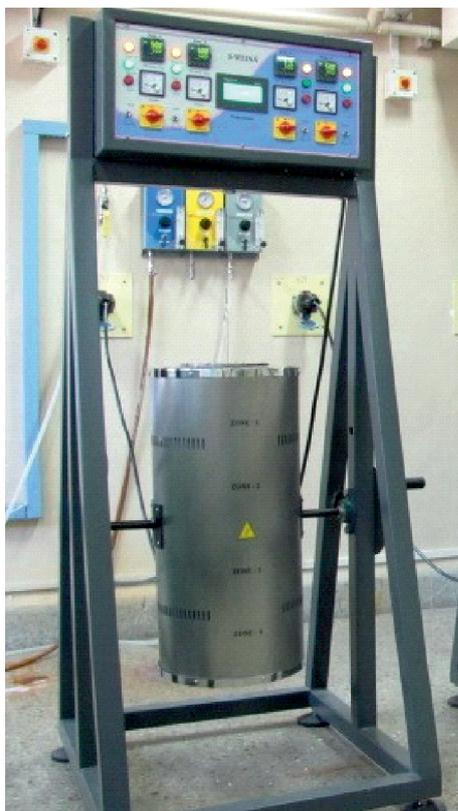
Fig.1: A typical Bridgman Crystal Growth Furnace.
