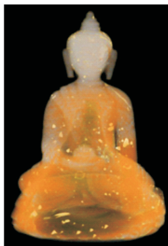
Neutron Tomography of Buddha relic: Wax remnants on surface due to bronze casting process were detected (last)
