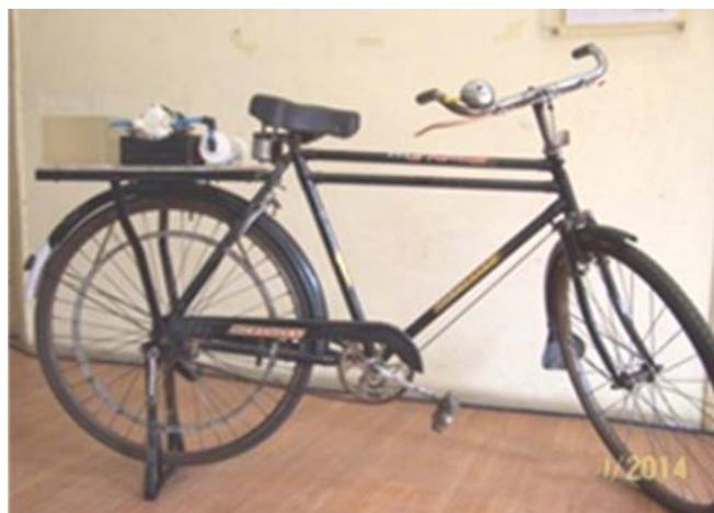
Fig. 8: Bicycle-mounted, foot/pedal operated RO / UF units
