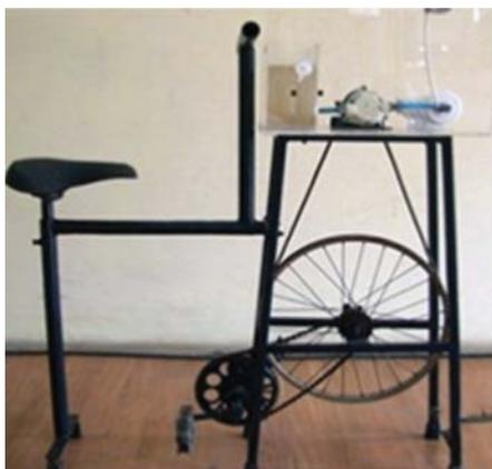
Fig. 7: Foot operated RO/UF units
