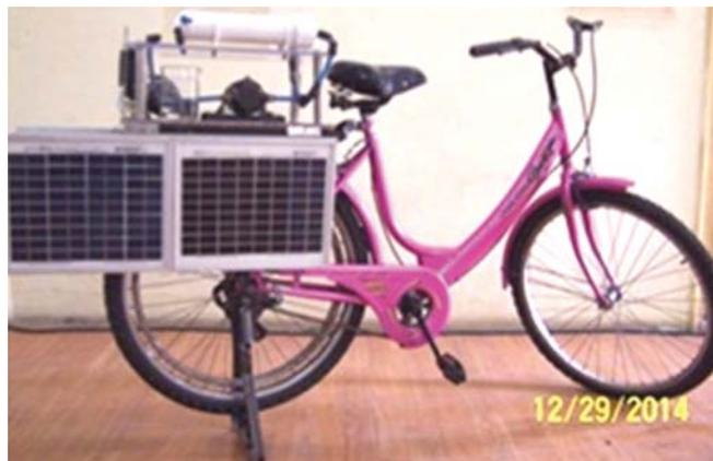
Fig. 9: Bicycle-mounted, RO / UF unit operated with hybrid power system
