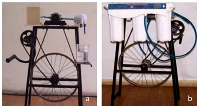
Fig. 6: (a) Capillary UF module (b) Multiple UF Candles
