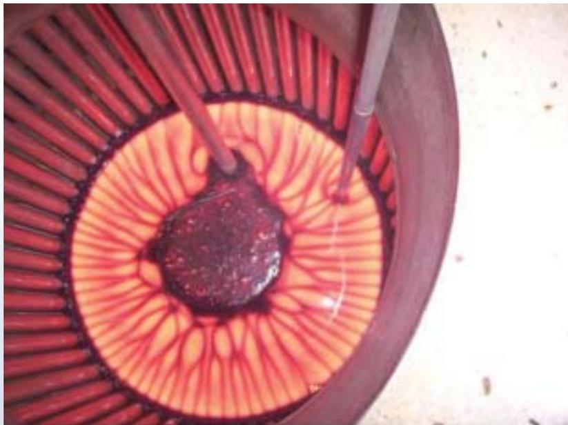
**Fig . 10 : Molten glass inside the engineering scale cold crucible**
