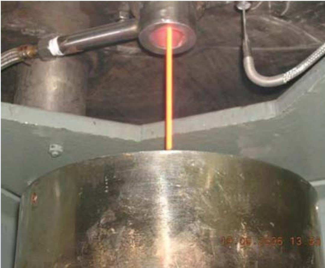
Fig. 11 : Glass pouring from the engineering scale cold crucible
