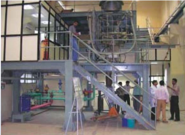
**Fig. 6 : Engineering scale demonstration facility for cold crucible induction melting**
