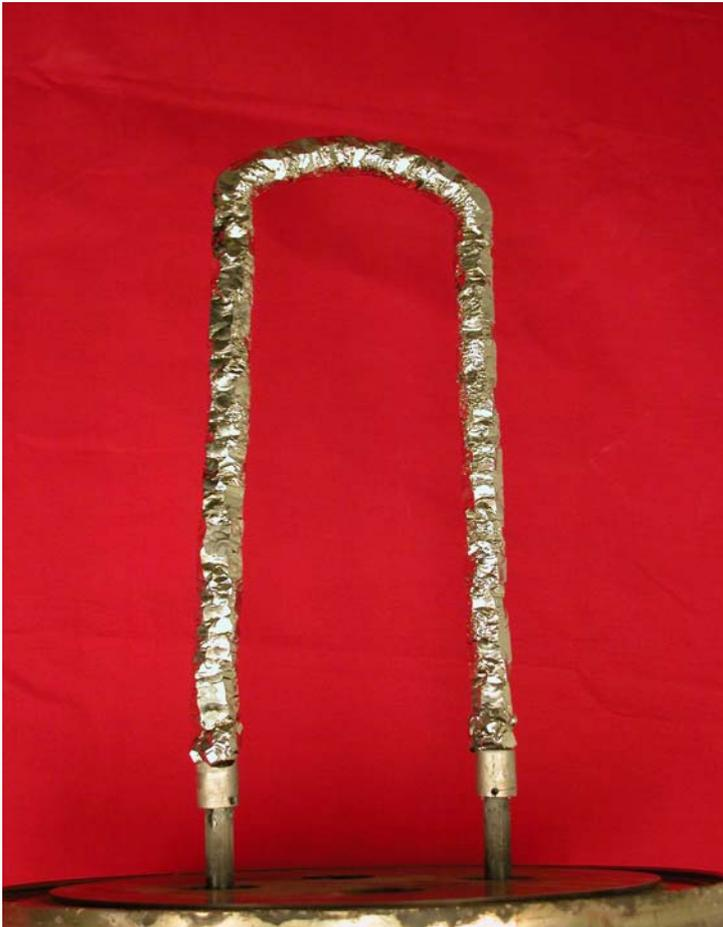
*Fig.5: Crystal bar zirconium with the retort cover flange (upside down)*
