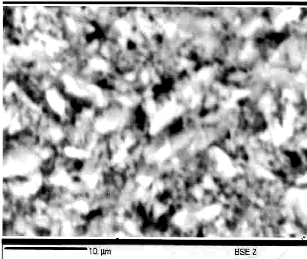
*Fig.2 SEM micrograph of DCS-20 pellet (bulk density 1.64 -1.72 g cm<sup>-3</sup>)*
