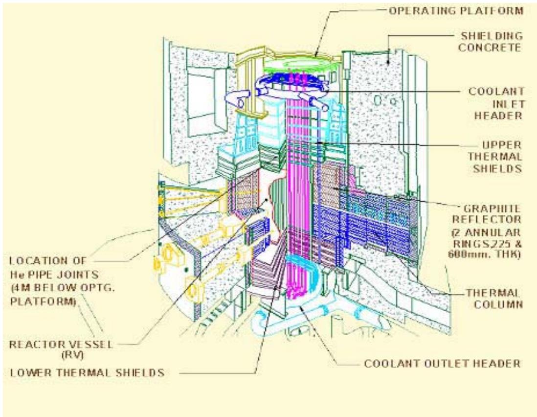
*CIRUS reactor structure cross section*
