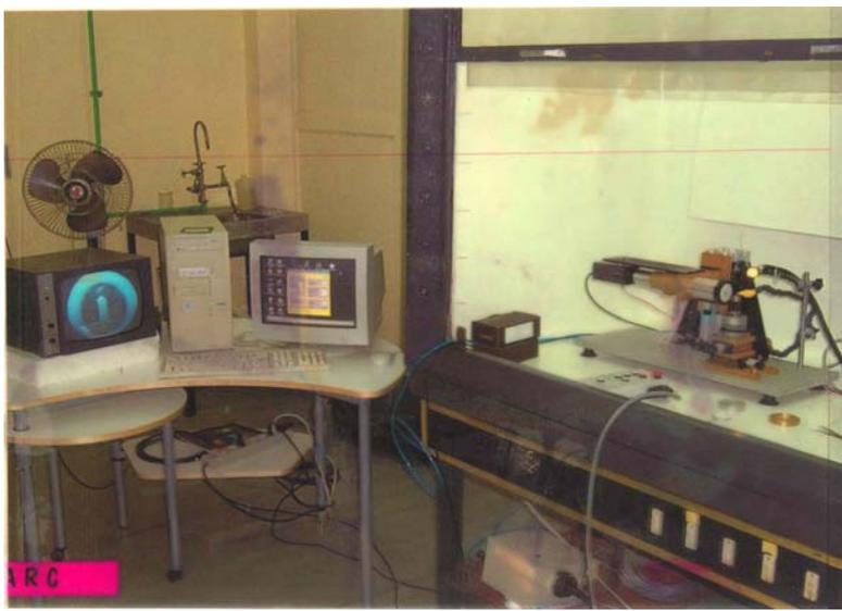
Fig. 5 Laser welding set-up inside a fume-hood
