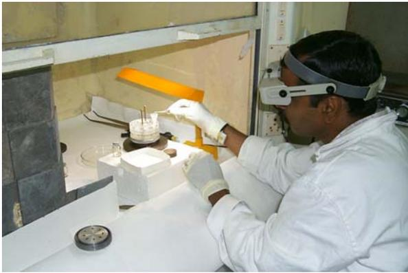
Fig. 6 Insertion of sources in capsules
