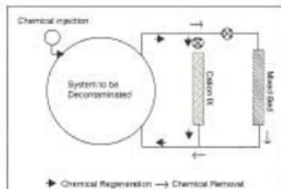
Fig. 1 Logistics of dilute chemical decontamination
