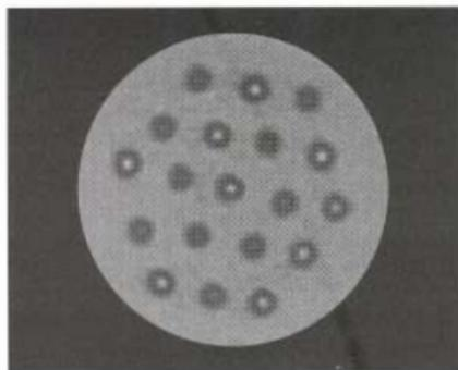
*Fig.9 Processed CT scan image to highlight differences of attenuation coefficient between SS and brass rods*
