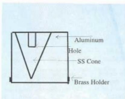
*Fig.10 Schematic diagram of test object with offcentered SS cone inside aluminum matrix*
