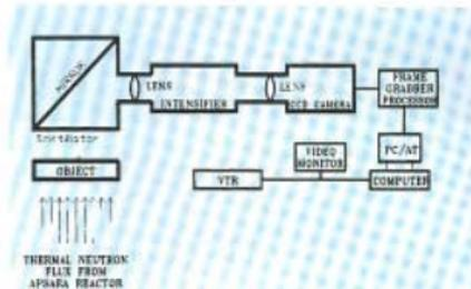
Fig.1 Schematic diagram of a prototype electronic imaging system at APSARA
