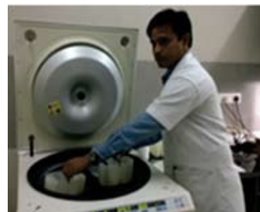
Centrifugation of whole blood in refrigerated centrifuge.
