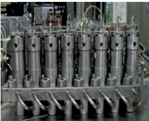
Centrifugal contactors used in CORAL plant
