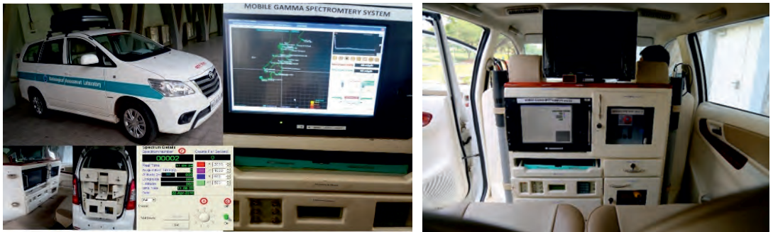
Fig.5: Mobile Radiological Assessment Laboratory with screen display during a survey
