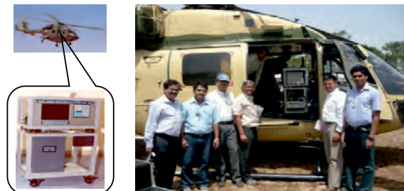
Fig.1: Aerial Gamma Spectrometry System (AGSS) developed and used by RSSD team in many aerial Gamma spectrometry surveys using helicopters and during mobile radiological surveys.
