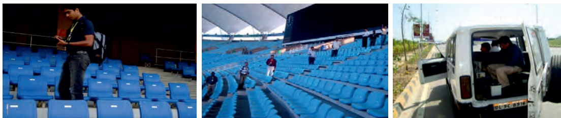
Fig.3: (a)'Source search' using 'Back Pack' Radiation Detection System, (b) monitoring of one of the stadia of CWG, (c) mobile monitoring of access roads to stadia
