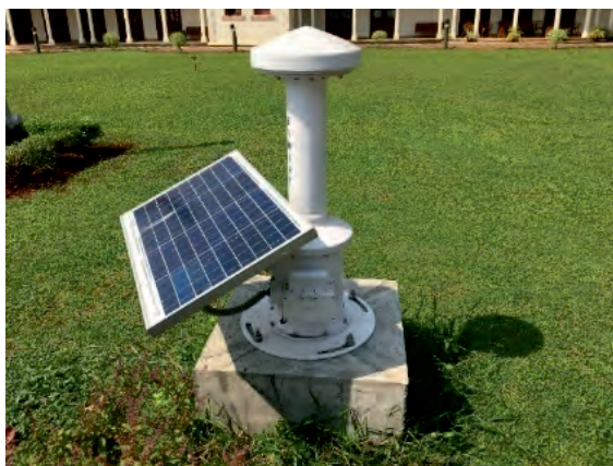
Fig.2: Environmental Radiation Monitor (ERM) of IERMON installed at one of the sites
