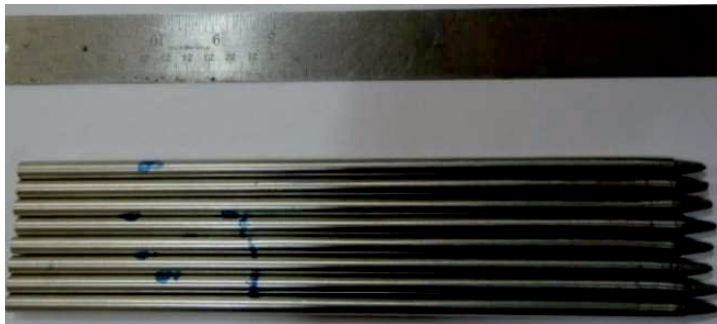
Figure 29.4. Magnetic pulse welded samples.
