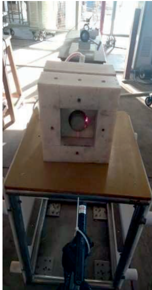
Figure 27.4. Set up for field measurement in Expansion EM Forming.
