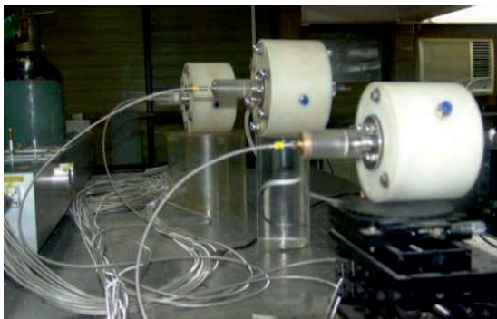
Figure 11.8(a). Photograph of sparkgaps assembly with focusing optics and (b). The output waveform of two switches showing jitter < 5 ns.
