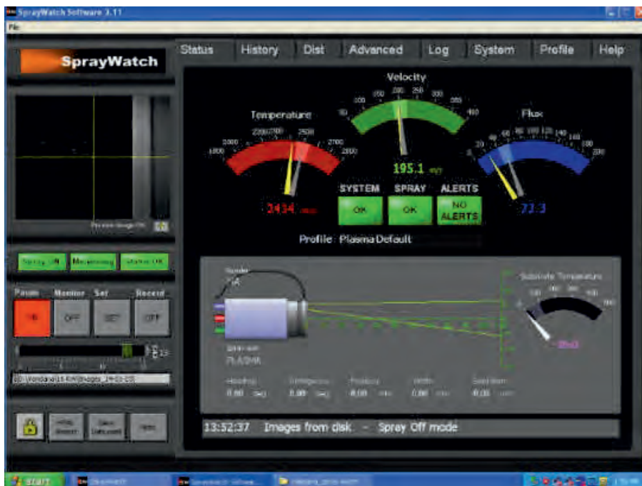
Figure 31.4: Spray watch experiment showing in-flight particle temperature and velocity.
