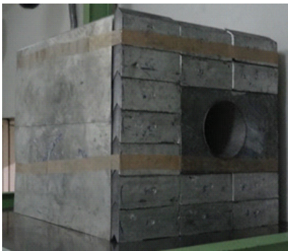
Figure 36.4: Photograph of photo-neutron target assembly setup used for neutron radiography.
