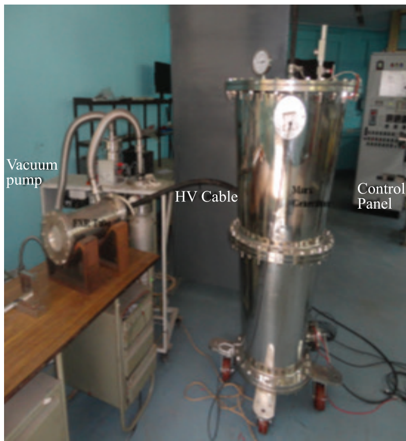
Figure 9.6: A photograph of the FXR system composed of the Compact Marx Generator, FXR Tube and the Control Panel.
