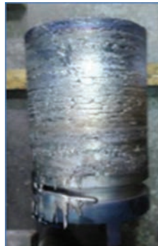
Figure 9.2: Electron beam melted Zirconium alloy (Courtesy: NFC, Hyderabad).
