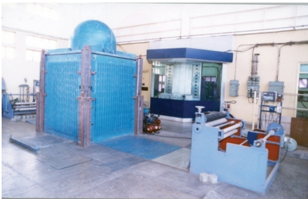
Figure 9.8: 500 keV DC Accelerator with shielding and product conveyor.
