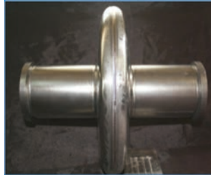
Figure 9.4: EB welded Niobium cavity.
