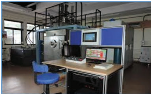
Figure 9.1: An Electron Beam welding machine uses electrons as energy carrier (photograph Ref: www.barc.gov.in ) [31].
