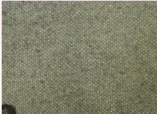
Electro-conductive cotton fabric prepared by electron beam induced graft polymerization and electroless deposition technology
