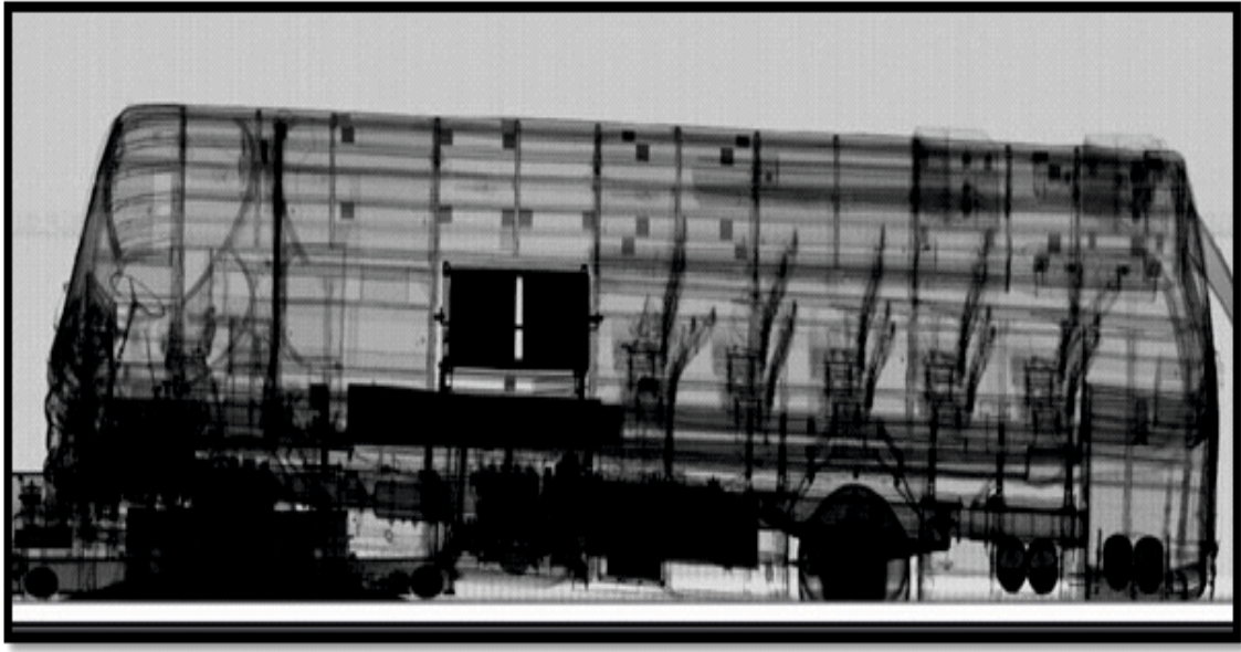
Imaging of Cargo at Gamma Field, BARC using 6 MeV System
